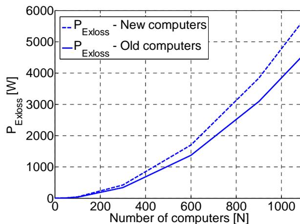
Fig. 7: Excessive losses determined for the “new” and “old” computers in the case of three-phase load.
