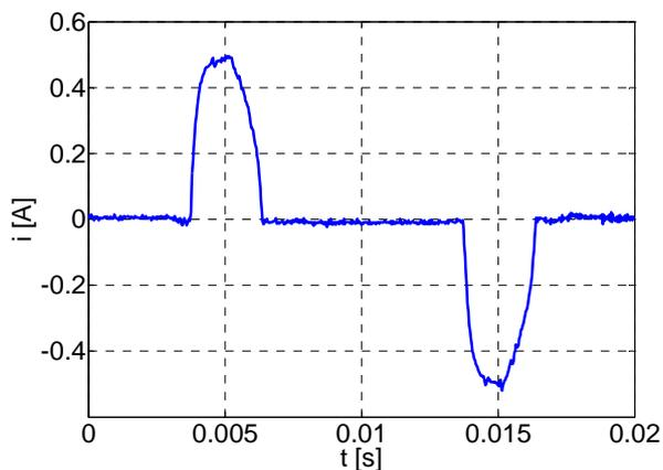
Fig. 4: Time dependent current signal of “old” computer.
