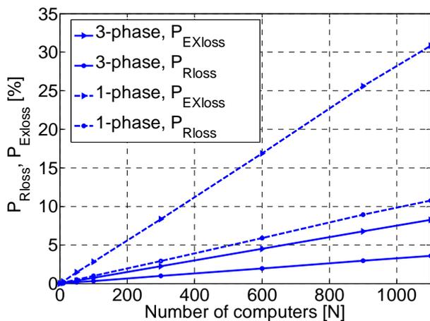
Fig. 8: Losses in low voltage cable which cannot be avoided and excessive transmission line losses for single-phase and three-phase systems.
