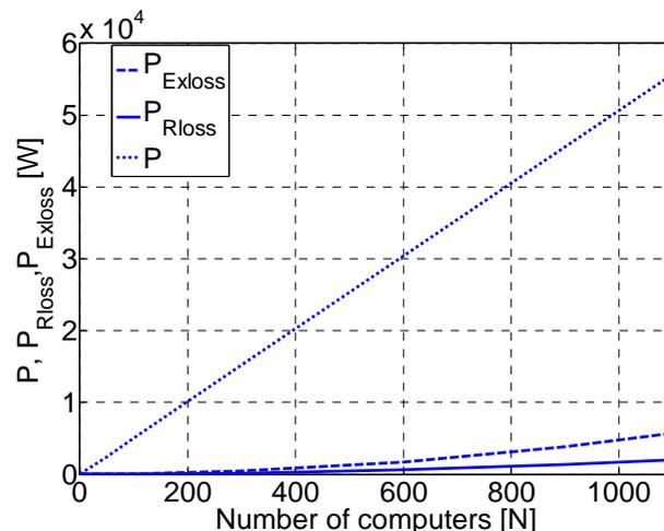
Fig. 6: Load power  $P$ , losses in low voltage three-phase cable which cannot be avoid  $P_{Rloss}$  and excessive losses  $P_{Exloss}$  caused by the nonlinear three-phase load.
