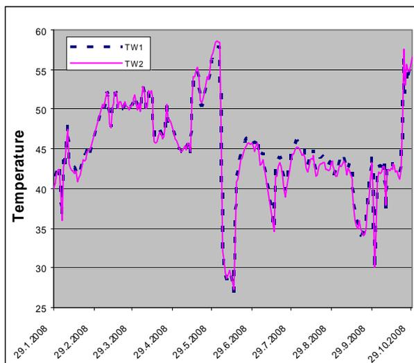
Fig. 3. Winding temperature in measurement interval from 29.1.to 29.10. 2008
