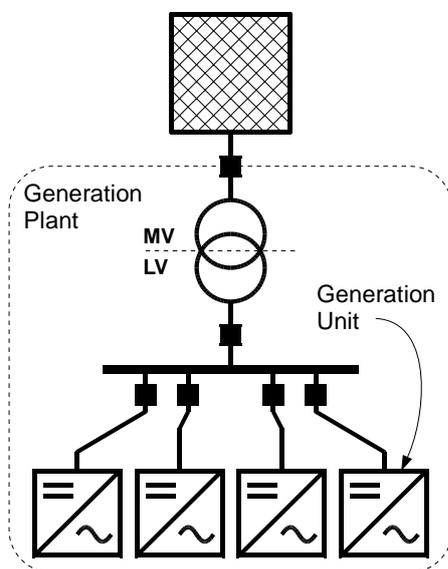
Fig. 1: Example of a generation plant connected to the medium voltage network composed of several generation units on the low voltage network.
