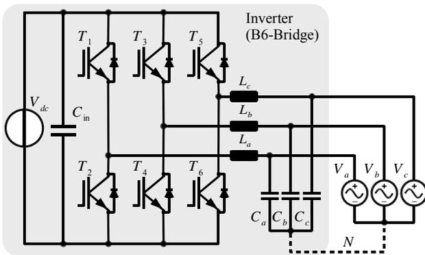
Fig. 5: A classic B6-Bridge VSI with a voltage input source.
