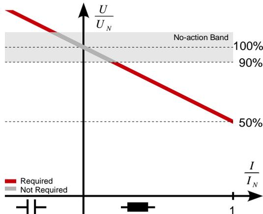
Fig. 3: Reactive current injection requirements
