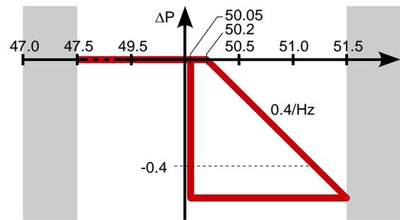
Fig. 4: Allowed frequency operating area and automatic active power throttling requirements.
