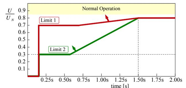
Fig. 2: Fault ride through requirements for generation units which are not based on direct-coupled synchronous machines.
