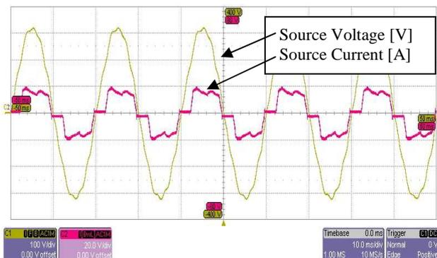
Fig. 3. Experimental results for source voltage ( $v_{sa}$ ) and source current ( $i_{sa}$ ) before filter operation.
