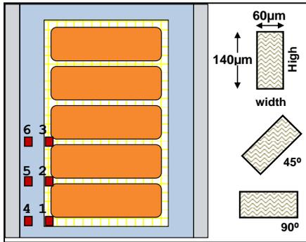
Fig. 3. Dimensions, location and orientation of the voids into the insulation systems (three different orientations per void were studied).
