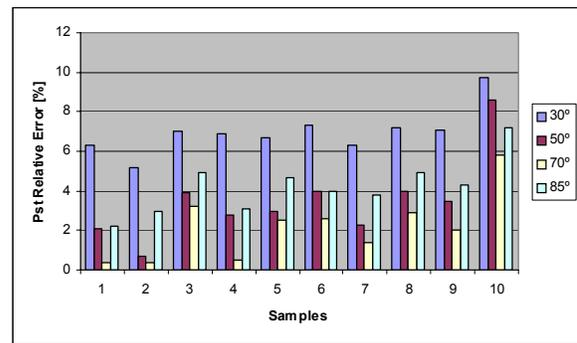
Fig. 3 –  $P_{st}$  relative error (%), continuous operation.
