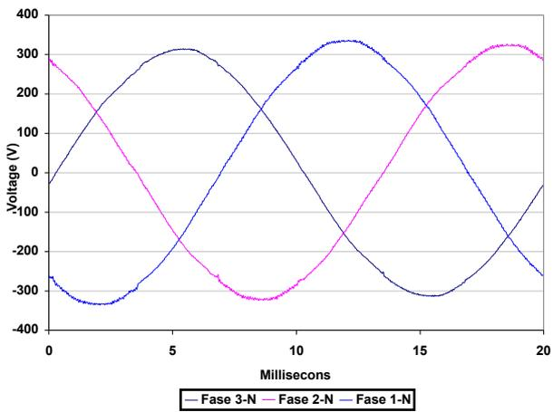
Figure 6. Voltage distortion at 28 kW<sub>e</sub>.
