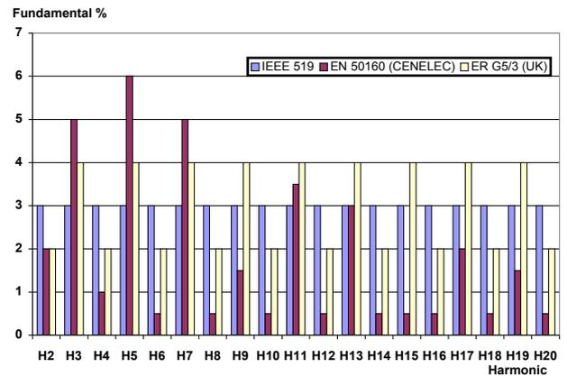
Figure 14. Some standards for voltage harmonics content.
