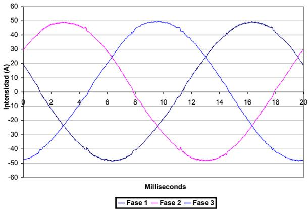
Figure 5. Current distortion at 24 kW<sub>e</sub>.
