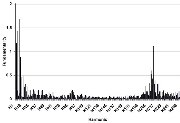
Figure 9. Voltage harmonic spectrum for 28 kW<sub>e</sub> Phase 2-N
