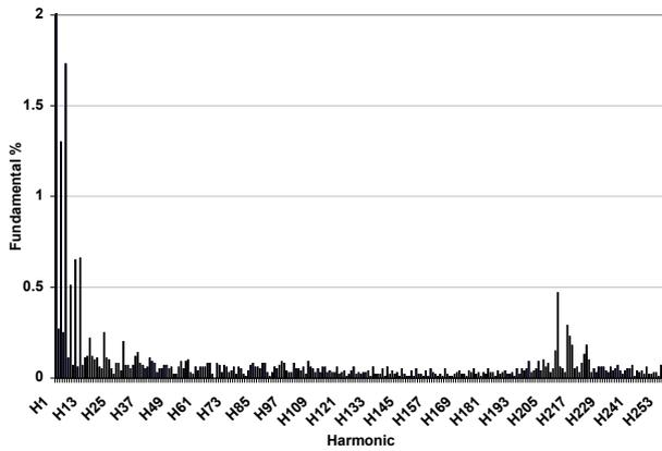
Figure 10. Voltage harmonic spectrum for 28 kW<sub>e</sub> Phase 3-N
