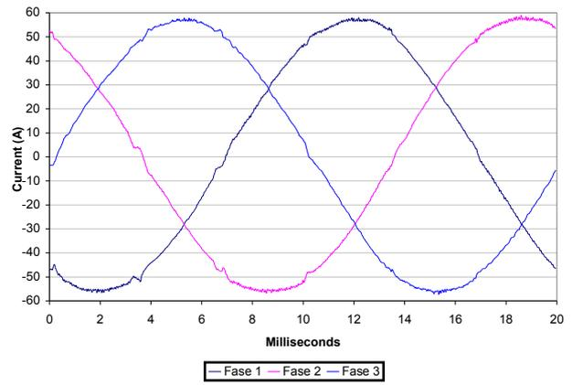
Figure 7. Current distortion at 28 kW<sub>e</sub>.
