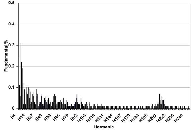
Figure 13. Current harmonic spectrum for 28 kW<sub>e</sub> Phase 3-N
