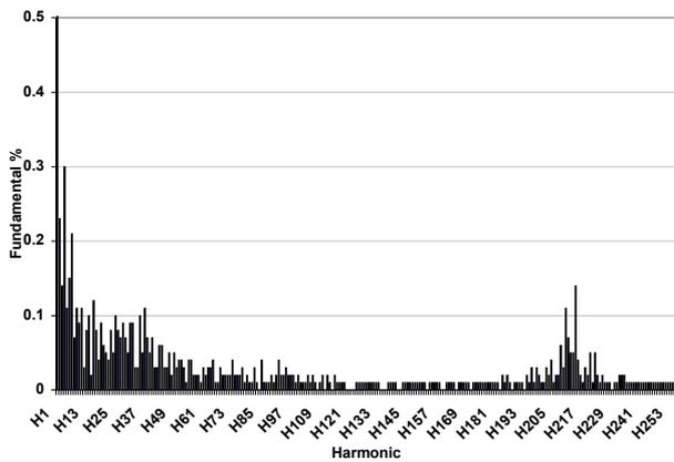
Figure 11. Current harmonic spectrum for 28 kW<sub>e</sub> Phase 1-N
