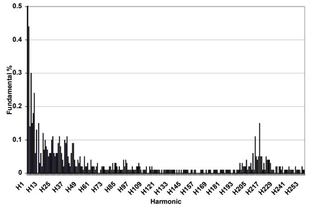
Figure 12. Current harmonic spectrum for 28 kW<sub>e</sub> Phase 2-N
