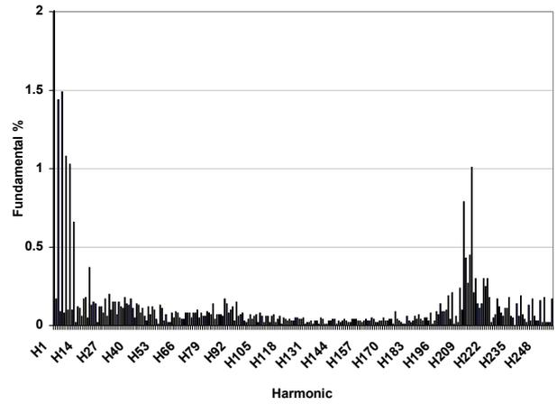
Figure 8. Voltage harmonic spectrum for 28 kW<sub>e</sub> Phase 1-N
