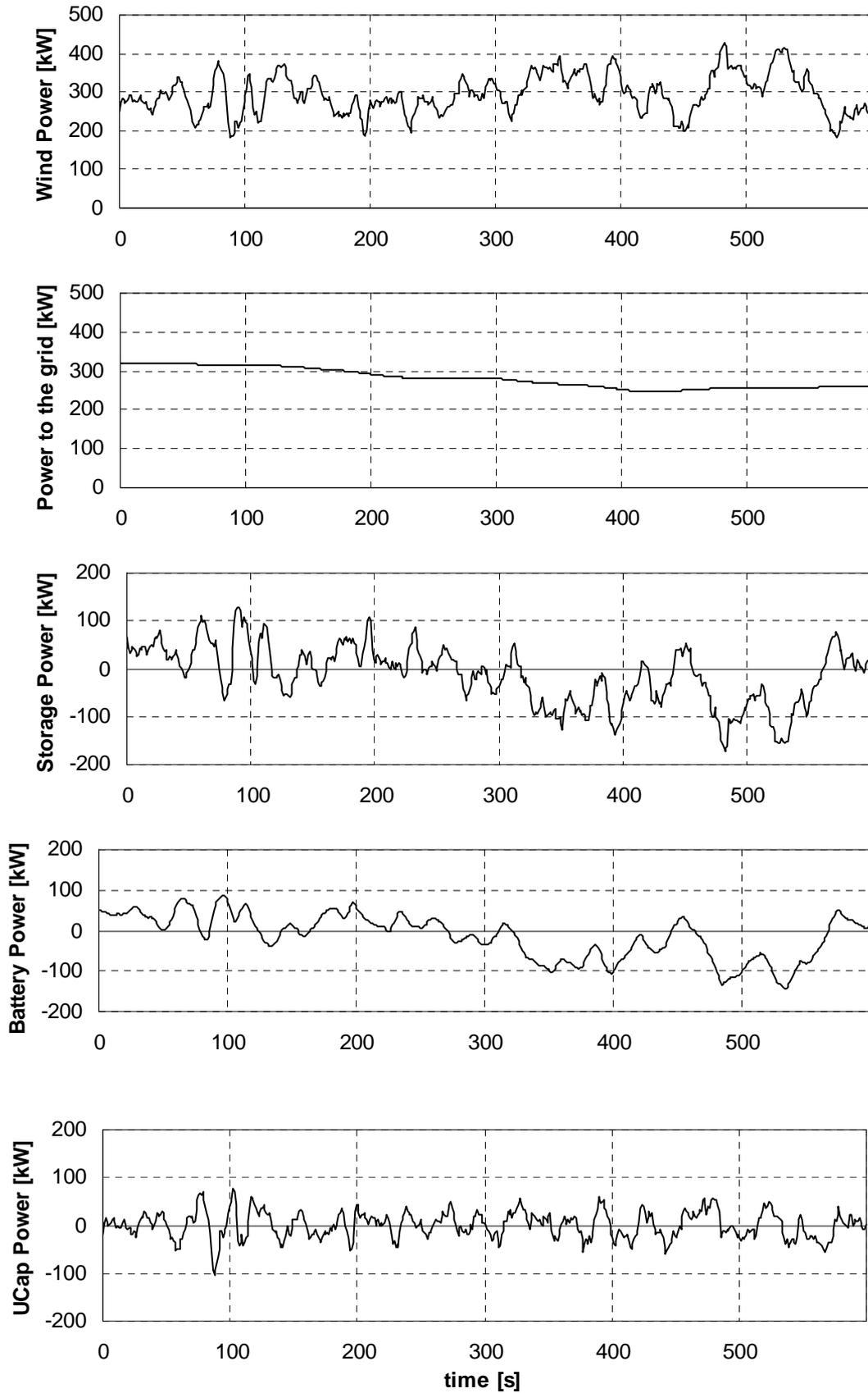
Fig. 3. Simulation results for the battery system with a 10 F ultra capacitor bank designed for a 10min time interval. From above: total input power to the storage system, input power to the battery, input power to the ultra capacitor bank.
