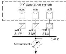
Fig. 1. Schematic view of 15 kW PV installation
