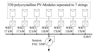
Fig. 2. Schematic view of 110 kW PV installation
