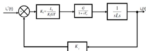
Fig. 6. Block schematic of the current control-loop
