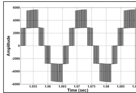
Fig. 4. Voltage waveform  $V_{AB} = V_{A1B1} + V_{A2B2}$  (i.e.  $V_r$ )
