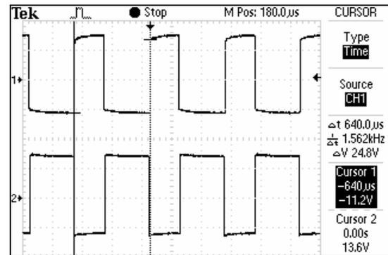
Fig. 26. Gate pulses for the same IGBTs of the same leg (Scale: X-axis: 1 division = 2 ms, Y-axis: 1 division = 10 V)
