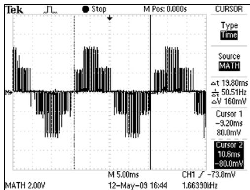
Fig. 31. Experimental waveform  $V_{AB} = V_{A1B1} + V_{A2B2}$  (i.e.  $V_f$ ) (Scale: X-axis: 1 division = 2 ms, Y-axis: 1 division = 10 V)
