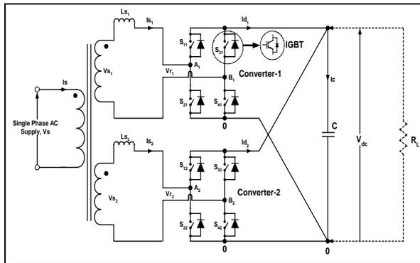
Fig. 2. Power Schematic of proposed front-end converter
