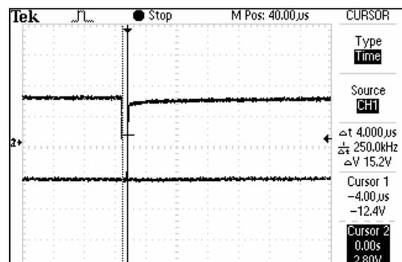
Fig. 28. Enlarged view of gate pulses for the IGBTs of the same leg showing dead-band (Scale: X-axis: 1 division = 2 ms, Y-axis: 1 division = 10 V)
