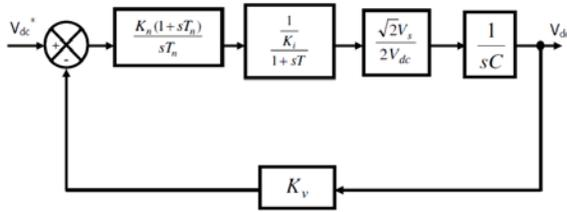
Fig. 7. Block schematic of the voltage control-loop
