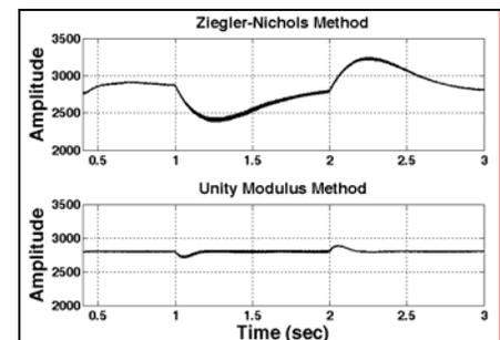
Fig. 13. Waveforms of dc-link voltage for over damped system during load change conditions
