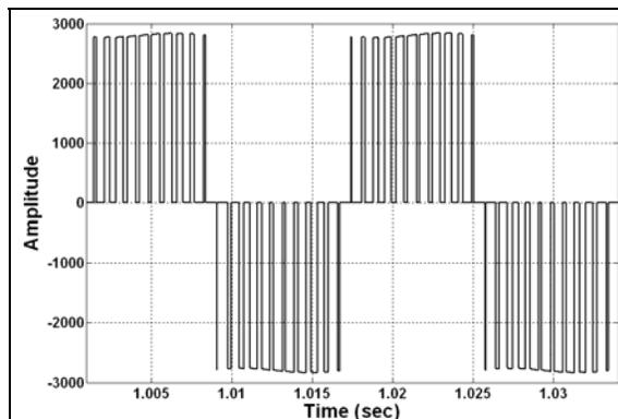
Fig. 3. Voltage waveform  $V_{A1B1} = V_{A10} - V_{B10}$  (i.e.  $V_{r1}$ )
