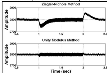
Fig. 11. Waveforms of dc-link voltage for under damped system during load change conditions
