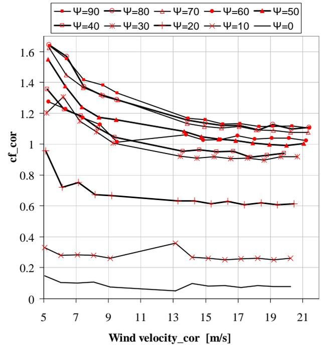
Fig. 8. Force coefficient with wind velocity correction
