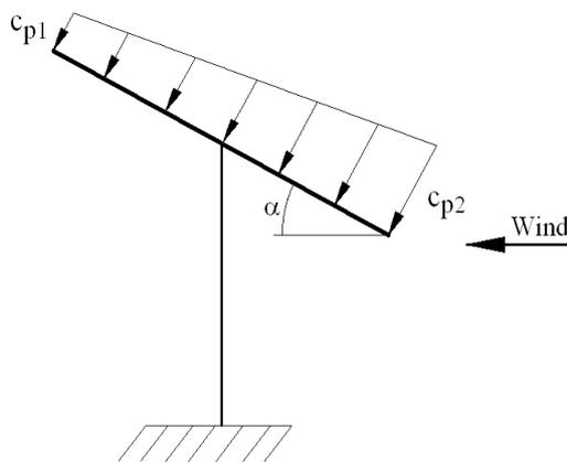
Fig. 3. Diagram of pressure coefficients distribution on tilted platforms [6]
