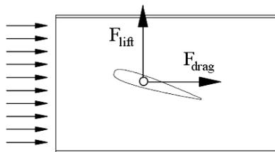
Fig. 5 Directions of the measured components
