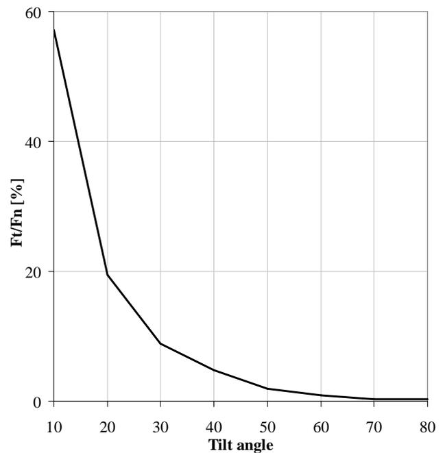
Fig. 12.  $F_t/F_n$  variation, depending on tilt angle
