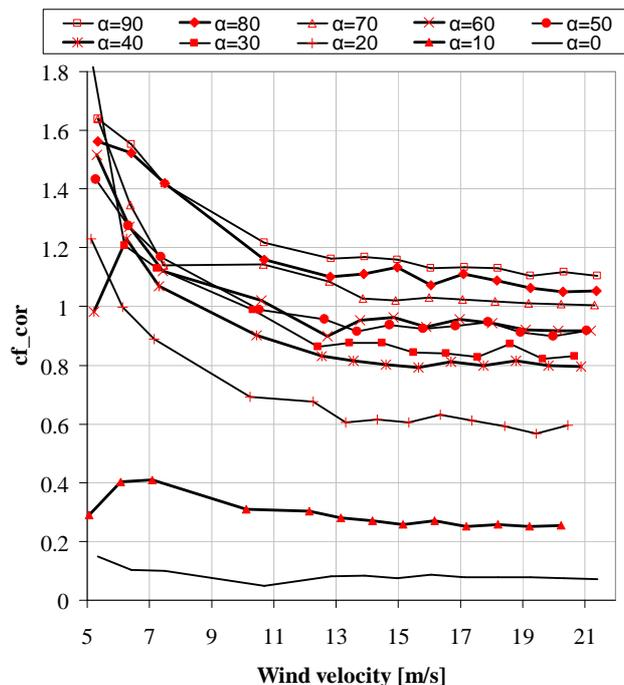
Fig. 14. Force coefficient with wind velocity correction
