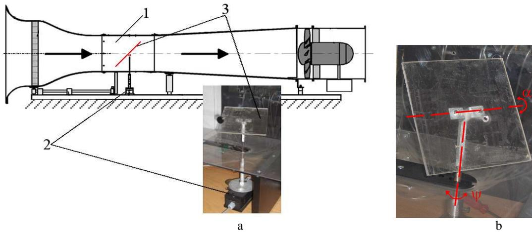
Fig. 4. Experimental stand and model
