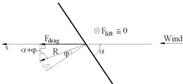
Fig. 13. Forces on the platform for altitudinal angle variation
