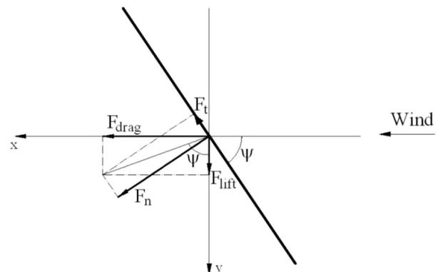
Fig. 6. Forces on the platform for azimuthal angle variation
