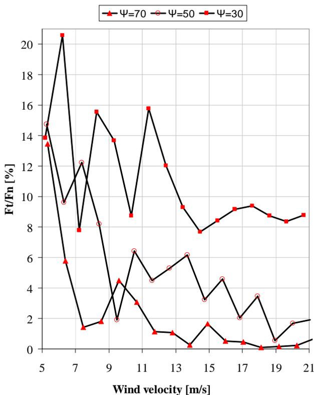
Fig. 11.  $F_t/F_n$  variation, depending on wind velocity
