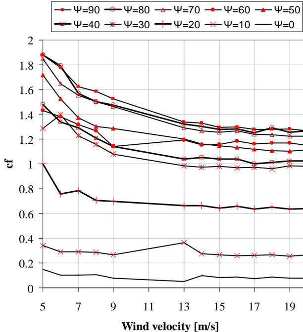
Fig. 7. Force coefficient without wind velocity correction
