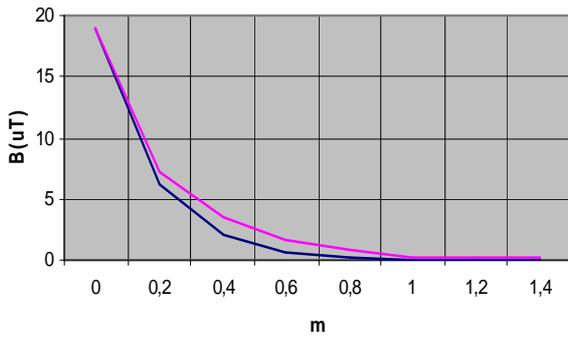
Fig. 2. Magnetic flux density versus distance in the case of the heating central
