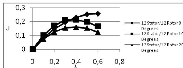
Figure.3 'Variation of power output with respect to  $\lambda$ '
