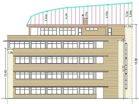
Outside the separation bubble, the wind speed increases. This increase is about 20% of the wind speed that corresponds to that height. The vector of wind velocity is not parallel to the roof but presents an angle with the horizontal plane, the separation angle. As a result, the acceleration vector of wind forms an angle of separation to the roof or to the sides of the building, which depends on the size of the building and the wildness or rugged of their surroundings.
