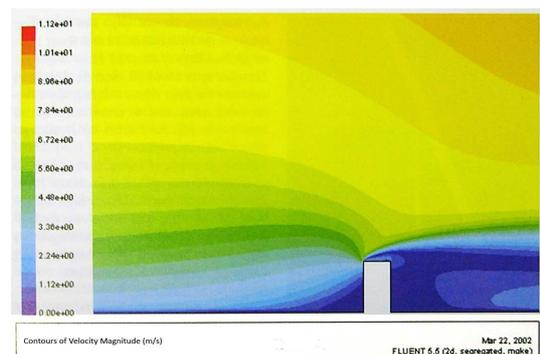
Next two images show, similarly to the previous one, the modification of the wind flow in a simulation obtained with FLUENT ©, but now in the vertical plane.
