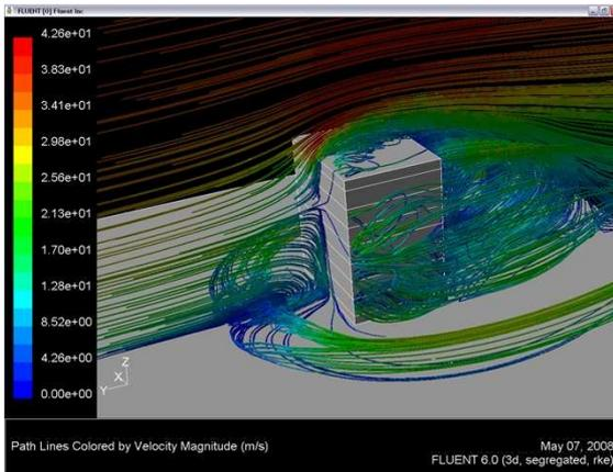
The wind flow separates at the edge of the roof of the building and forms a low speed separation bubble.
