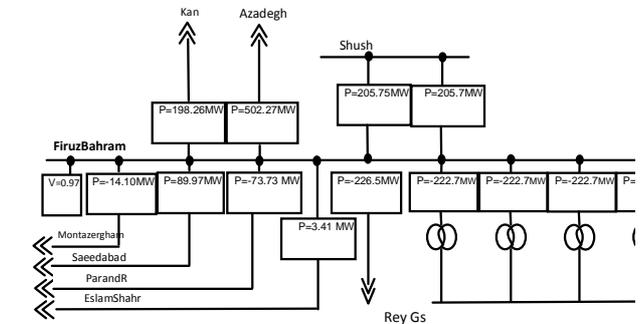
Fig. 3. Load flow analysis in Firuzbahram 400/230 kV substation
