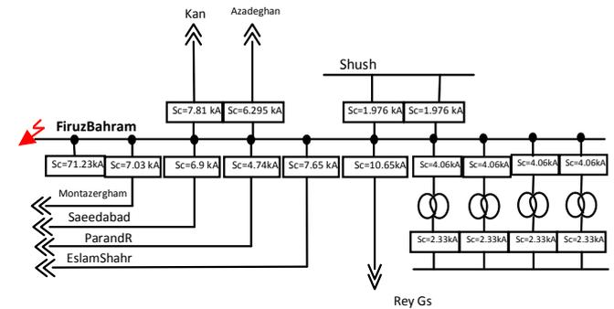
Fig. 2. SC analysis in Firuzbahram 400/230 kV substation
