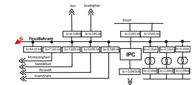
Fig. 4. SC analysis in Firuzbahram substation with IPC installed in "Firuzbahram – Rey Gs" 230 kV line
