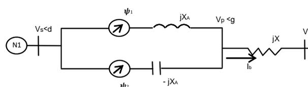
Fig. 1. IPC in series with a transmission line
