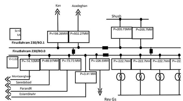
Fig. 5. Load flow analysis in Firuzbahram substation in double busbar configuration without using IPC
