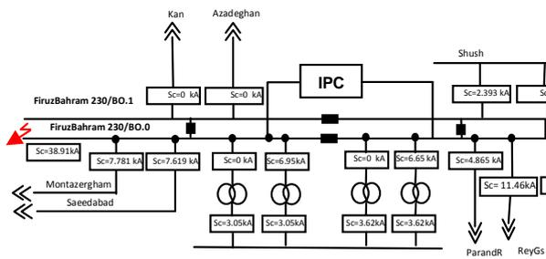
Fig. 6. SC analysis in Firuzbahram substation with an IPC used as a bus splitting device
