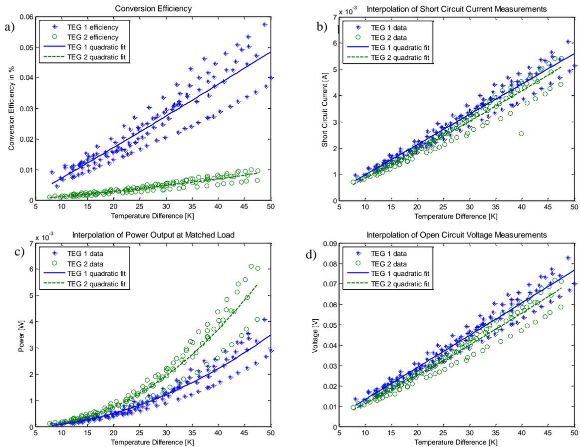
Fig. 5. Measurements of TEG 1 (stars) and TEG 2 (circles), each plot with least square quadratic fittings, continuous line for TEG 1, dashed for TEG 2.
