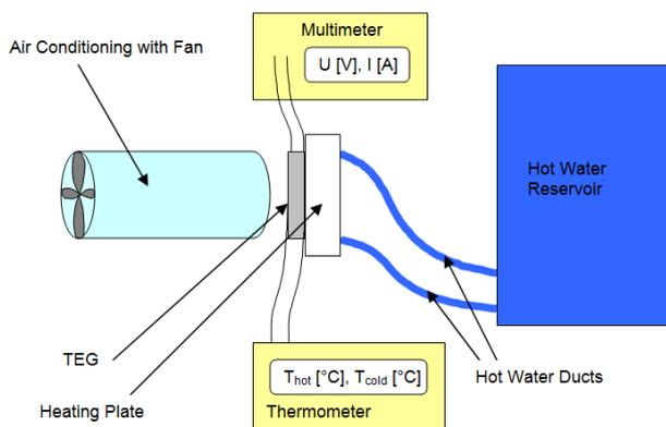
Fig. 1. Experimental Setup for thermoelectric generator measurements.
