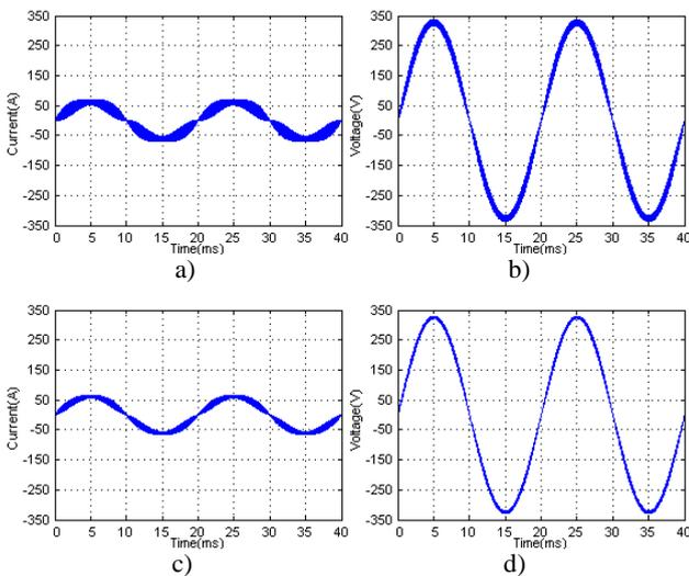
Fig. 6. a) Inductor current and b) output voltage when three-level full bridge is connected to 750 V DC and  $THD_u$  is  $\leq 5\%$ , c) inductor current and d) output voltage when three-level full bridge is connected to 750 V DC and  $THD_u$  is  $\leq 2\%$
