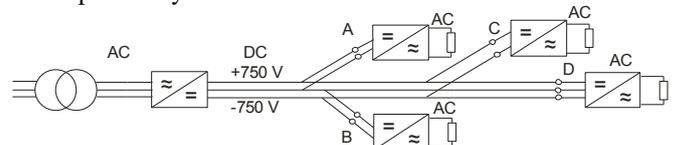
Fig. 2. A bipolar LVDC distribution network
