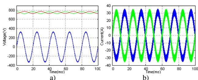
Fig. 7. a) Output voltage, voltages of the DC link capacitors and b) currents of the DC link capacitors when two-level half bridge is connected to 1500 V DC
