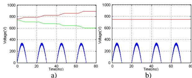
Fig. 8. Load voltage and voltages of the DC-capacitors when a) three-level half-bridge and b) three-level full bridge supplies half-wave rectifying load
