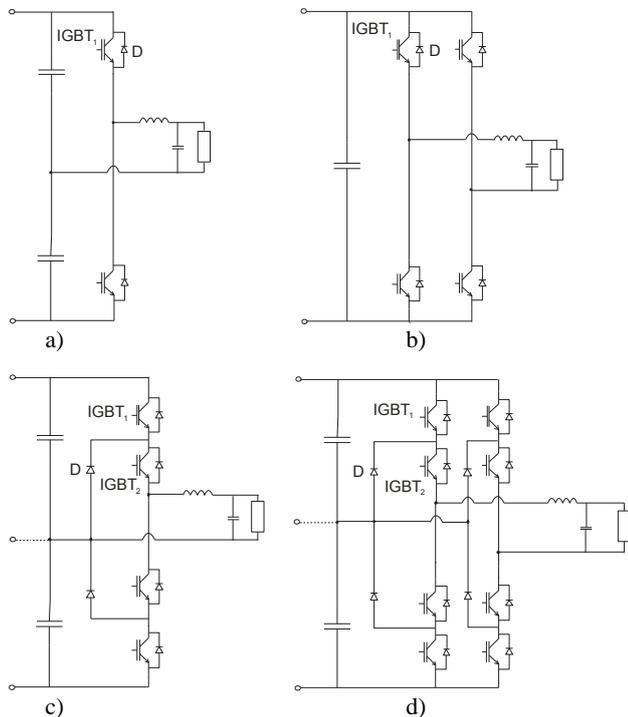
Fig. 3. Single-phase two-level a) half bridge, b) full bridge and three-level c) half bridge, d) full bridge
