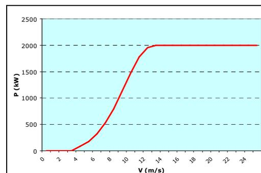
Figure 7. 2 MW Wind turbine power curve.
