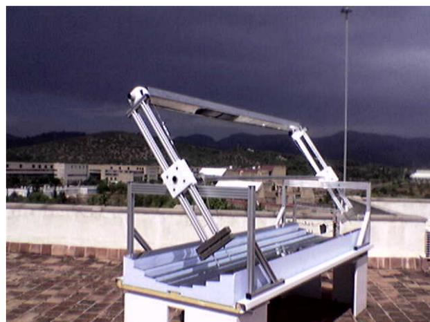
Figure 11. Solar Collector with static reflector
