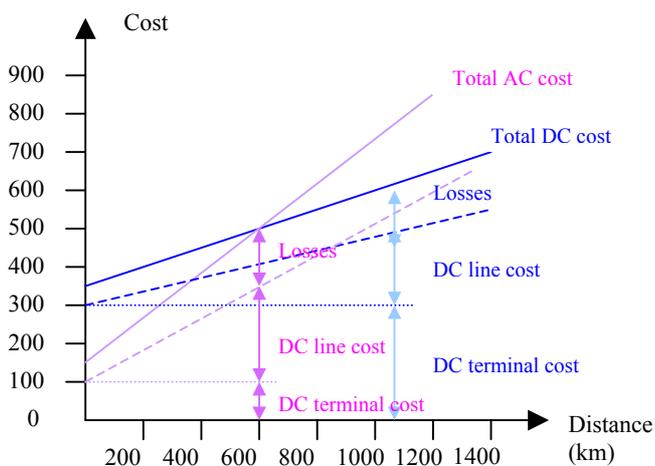
Fig. 3. HVAC-HVDC cost
