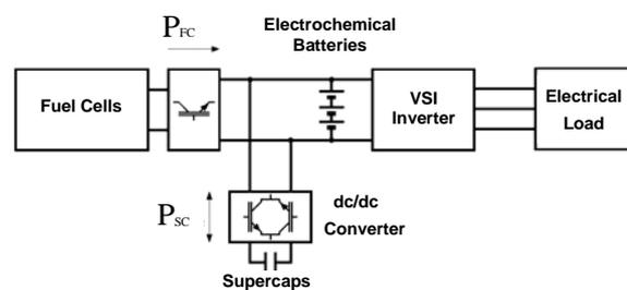
Fig.2 – Block scheme of a compound storage system
