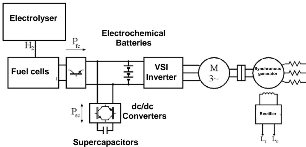
Fig.5 – Block diagram of the drive used for experimental tests
