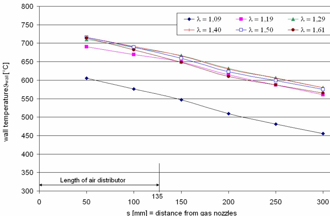
**Figure 7:** Temperature of combustion chamber wall for the gas mixture from biomass gasification at 30 kW<sub>th</sub>
