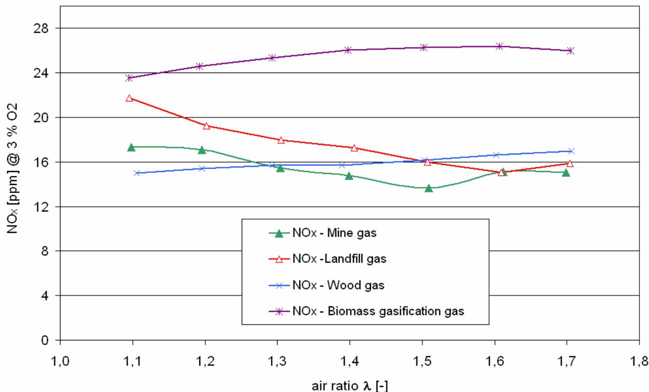
**Figure 3:** Measured  $NO_x$  emission values at 30 kW<sub>th</sub> for different low calorific gas mixtures
