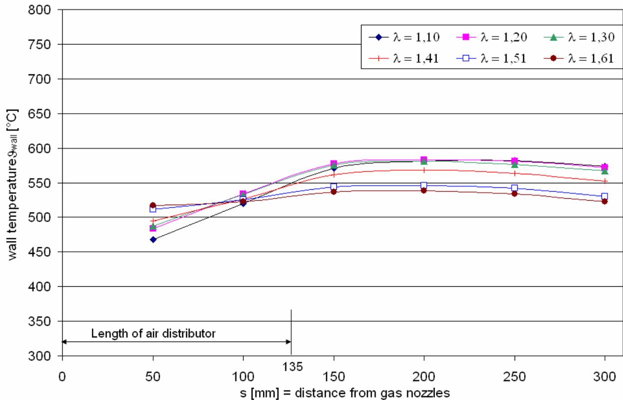
**Figure 8:** Temperature of combustion chamber wall for the landfill gas mixture at 30 kW<sub>th</sub>
