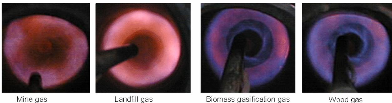
**Figure 6:** Flame photographs of COSTAIR burner for different low calorific gases at 30 kW<sub>th</sub>
