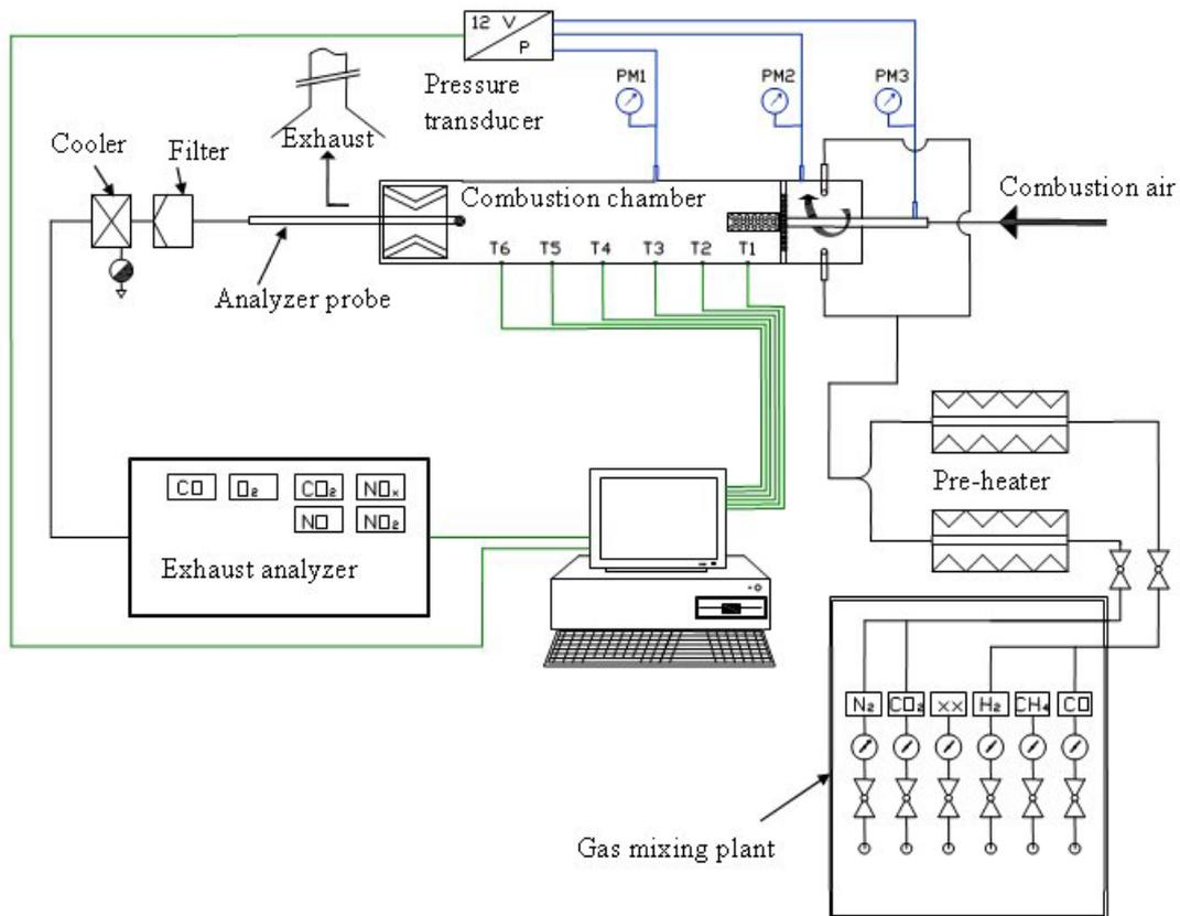
Figure 2: Schematic presentation of GWI test rig
