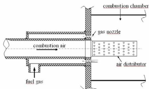
Figure 1: Design of the COSTAIR burner
