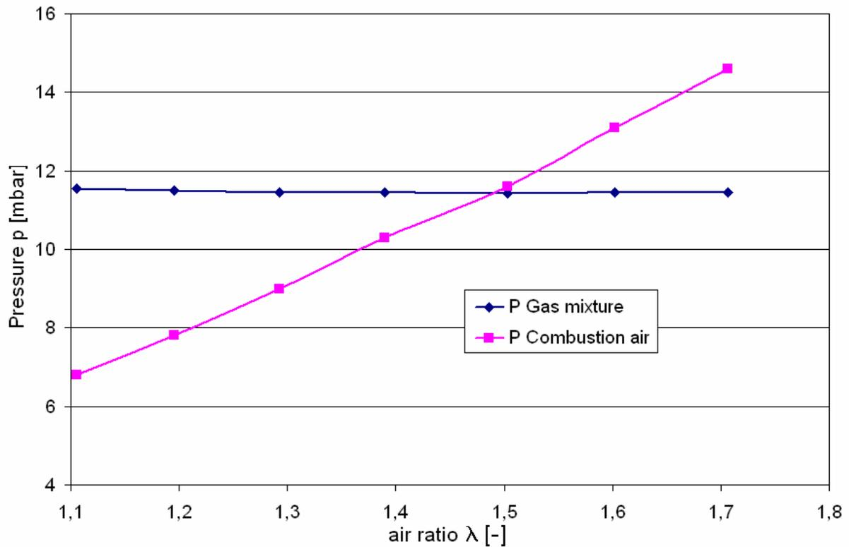
**Figure 5:** Measured pressures at 30 kW<sub>th</sub> for wood gas mixture and combustion air
