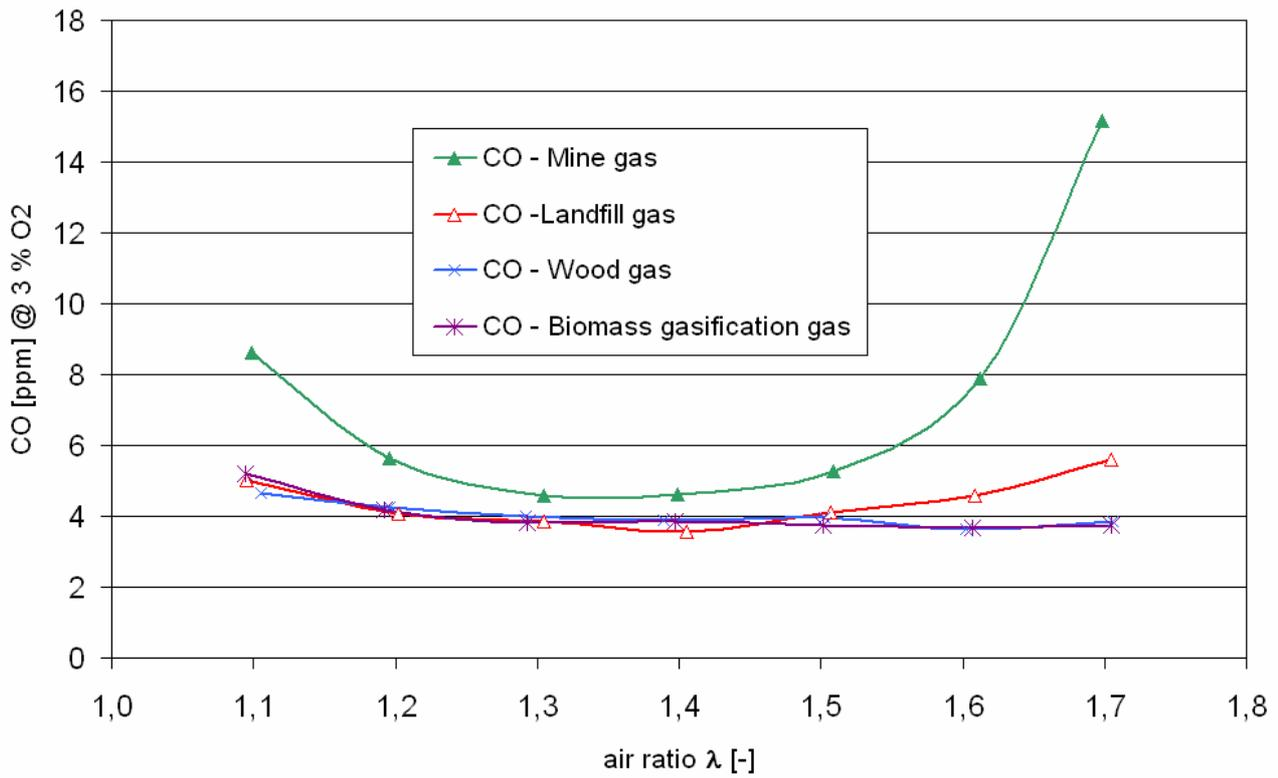
**Figure 4:** Measured CO emission values at 30 kW<sub>th</sub> for different low calorific gas mixtures
