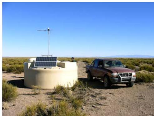
View 1: A Pierre Auger Čerenkov tank. In detail the PV modules
