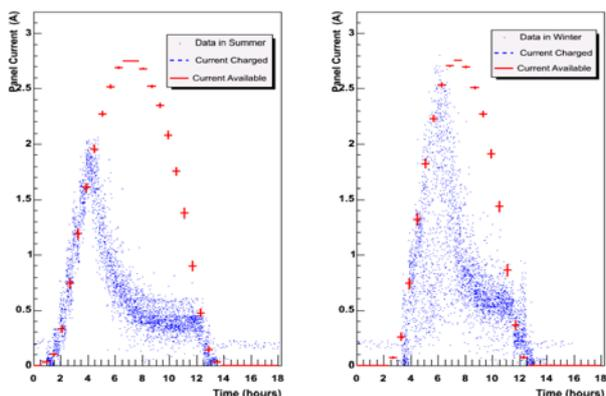
Fig. 3. In the left, photovoltaic module's current and batteries input's one (blue) versus time in summer. The right figure shows the same in winter.
