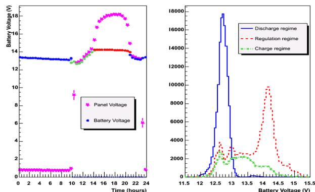
Fig. 1. Left: voltage values throughout a day for photovoltaic modules (empty and pink) and batteries (rest). Right: the corresponding voltage distribution functions. Each performing regime is in a different colour.
