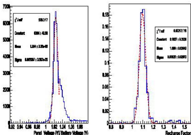
Fig. 2. In the left, the rate between the panel voltage and the batteries ones. The right figure shows the Charge Factor distribution throughout a year.
