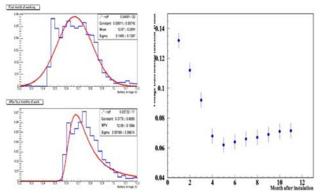
Fig. 2. Left: discharge distribution of a sample of batteries recently installed (adjusted with a Gaussian) and after 4 months of use (adjusted to a Landau distribution). Right: width of the voltage distribution in discharge regime throughout the first year of life in a sample of 100 batteries.
