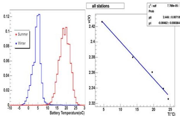
Fig. 4. In the left, temperature distribution in extremes (winter: blue, summer: red) Right, each cell's voltage dependence in discharge mode by temperature.
