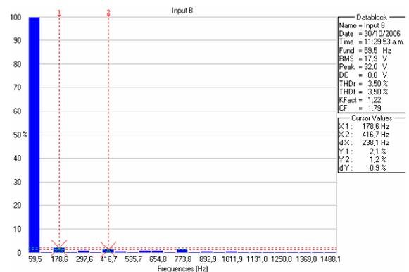
Fig. 18. Harmonic Spectrum of the Output AC Voltage.
