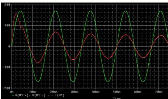
Fig. 10. Input current (red trace) and input voltage (green trace) for a full load (1200W).
