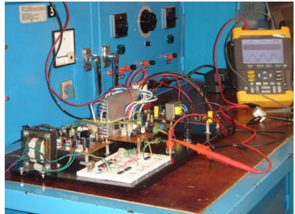
Fig. 16. Power stage of the full bridge inverter.
