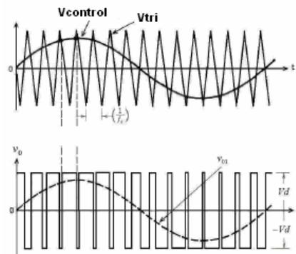
Fig. 7. PWM with Bipolar Switching.
