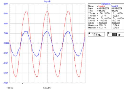
Fig. 12. Input voltage (red trace) and input current (blue trace).
