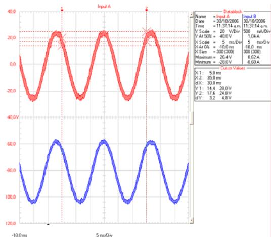
Fig. 17. Output AC Voltage and AC Current.
