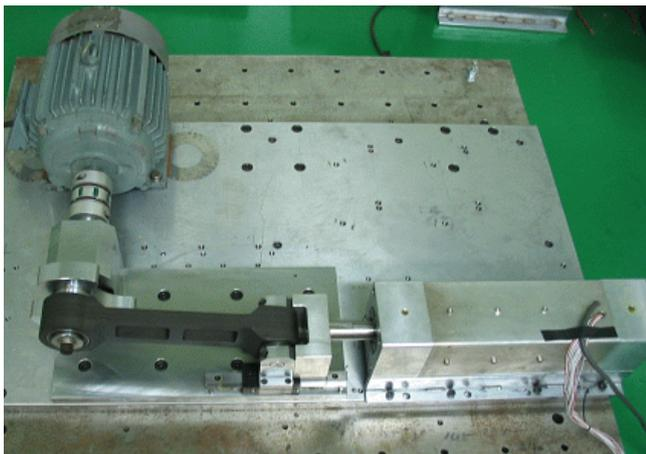
Fig. 10. Assembled linear generator and experimental setup.
