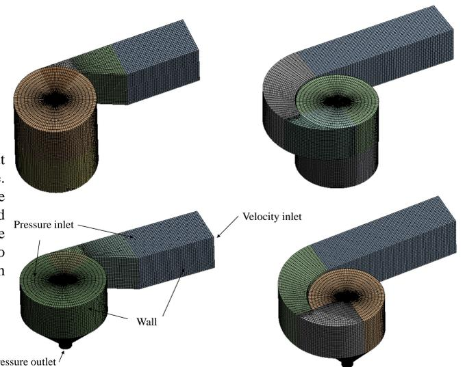
Figure 3. Computational domain of the inlet channel and basin. a) Tangential inlet with cylindrical basin, b) surrounding inlet with cylindrical basin, c) tangential inlet with conical basin, d) surrounding inlet with conical basin.
