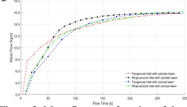
Figure 2. Mass flow as a function of the time.
