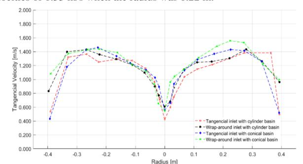
Figure 6. Tangential velocity distribution along the radial direction for several basins and inlets.
