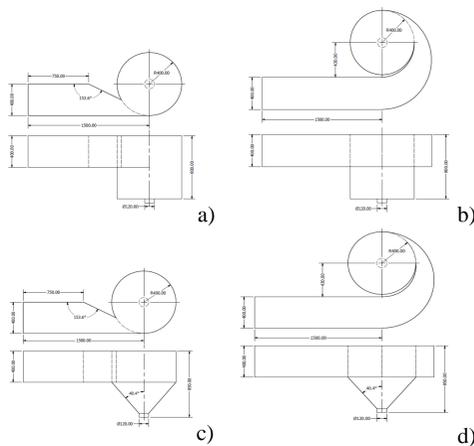
Figure 1. Geometrical configuration of the inlet channel and basin. a) Tangential inlet with cylindrical basin, b) wrap-around inlet with cylindrical basin, c) tangential inlet with conical basin, d) wrap-around inlet with conical basin.
