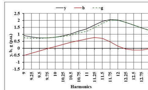
Fig. 2. Frequency responses on the 9-13-th harmonics in the node 2401
