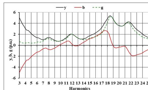
Fig. 1. Frequency responses on the 3-25-th harmonics in the node 2401
