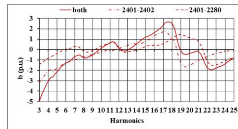
Fig. 3. Frequency response of susceptance for node 2401
