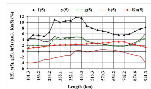
Fig. 5. Parameters of nodes and modes of 220 kV network on the 5-th harmonic
