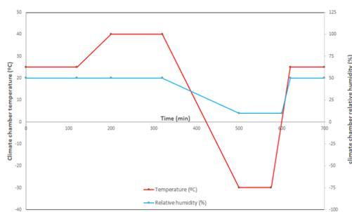
The stack was subjected to a very long term climate test, by following the temperatures and relative humidity according to the temperature and HR profile shown in the picture at the left.
