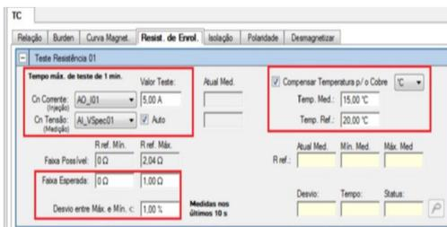
Fig. 3. Adjustments for winding resistance test
