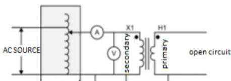
The test is performed in the secondary, due to the small current value that needs to be applied, since this winding works with a higher voltage level. This situation is preferable, because the limiting factor for this case is the insulation of the equipment, which does not change its size. [12,13].
