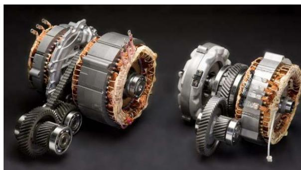
Figure 1. Ensemble MG1-MG2-Transaxle of 1997 (left) and 2004 (right) Toyota Prius.
