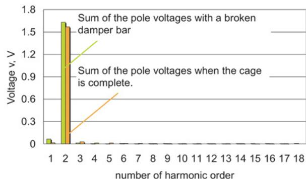
Fig. 9. Fourier analysed sum of the pole voltages
