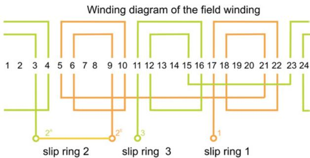
Fig. 6. Winding diagram of the distributed field winding of the test machine
