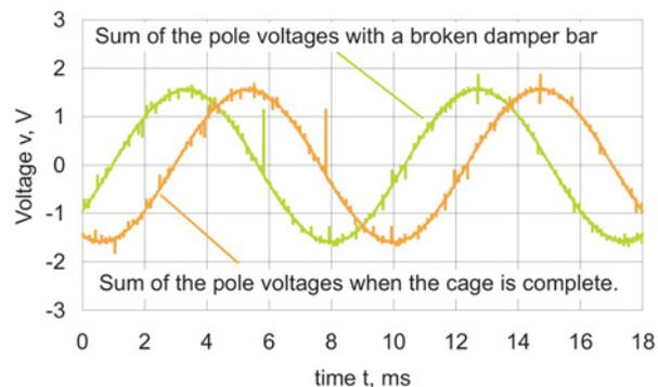
Fig. 8. The sum of the pole voltages when the machine is error free and when the machine has a broken bar.
