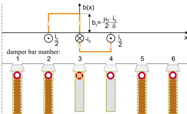
Fig. 1. Idealised interference field distribution
