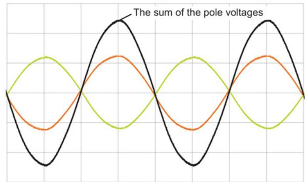
Fig. 5. The sum voltage of the pole voltages when the bar with the number 1 is broken
