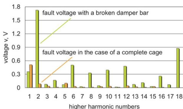
Fig. 11. Fourier analysed difference voltage of the synchronous machine (error-free and defected)
