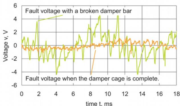
Fig. 10. The difference voltages of an error-free machine and a defected machine when the machine works in the lock mode.
