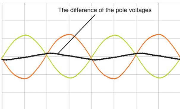
Fig. 4. The difference voltage of the pole voltages when the bar with the number 1 is broken
