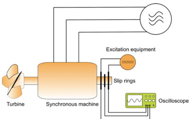
Fig. 7. The measuring circuit of the test machine
