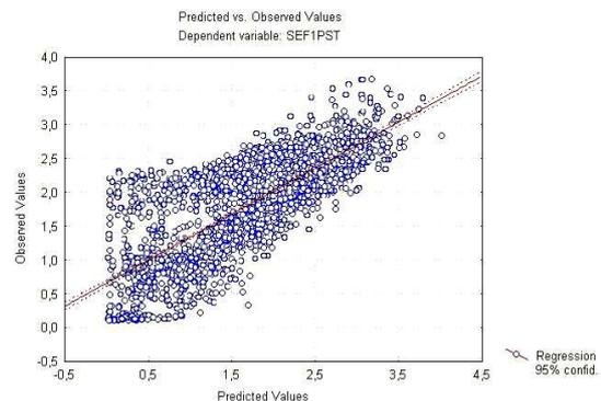
Figure 6 – Result of linear regression of the flicker P<sub>st</sub> at the substation in the corresponding values from the two wind turbines
