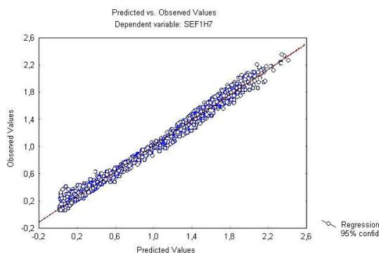
Figure 5 – Result of linear regression of the 7<sup>th</sup> harmonic at the substation in the corresponding values from the two wind turbines
