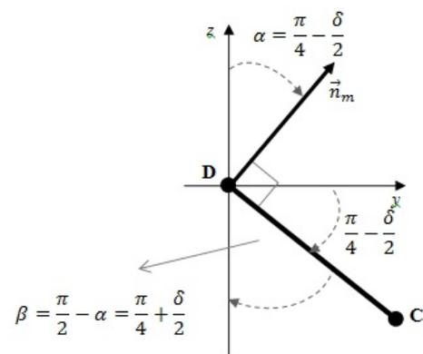
Fig. 3. Angles between the normal vector of the mirror and the Earth's rotation axis.
