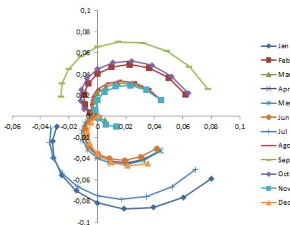
Fig. 7. Trajectories of incidence point for the 15<sup>th</sup> of each month respect the target point. Coordinates are given in m.
