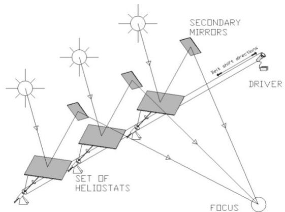
Fig. 5. Proposal of association of several devices to be moved with a unique engine and of the use of secondary mirrors.
