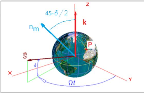
Fig. 1 Considered vectors for the proposed heliostat in an equatorial reference system.
