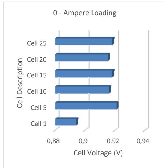
Figure 5. Ballard Mark 9™ cell to cell variation at OCV.
