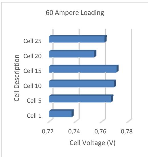
Figure 8. Ballard Mark 9™ cell to cell variation at 60 amps.
