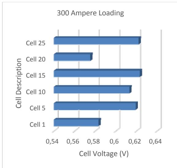
Figure 11. Ballard Mark 9™ cell to cell variation at 300 amps.
