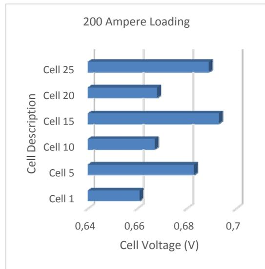
Figure 10. Ballard Mark 9™ cell to cell variation at 200 amps.
