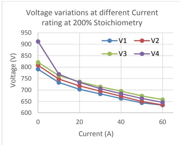
Figure 2. Cell voltage variation from OCV- 60A load for the 4 cell stack at 200% air Stoichiometry
