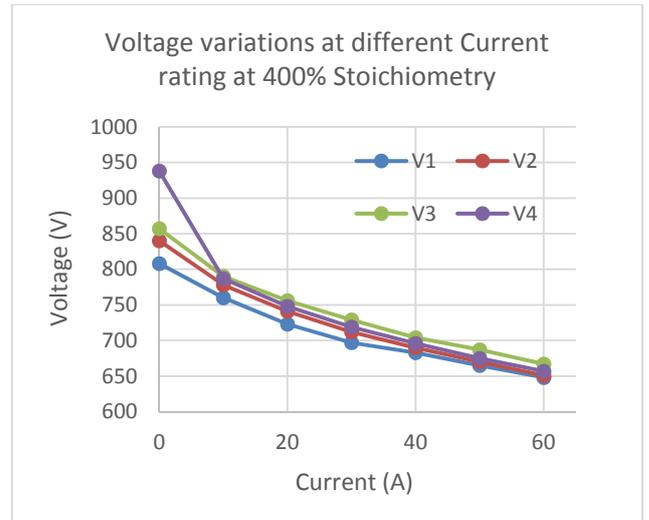
Figure 4. Cell voltage variation from OCV- 60A load for the 4 cell stack at 400% air Stoichiometry
