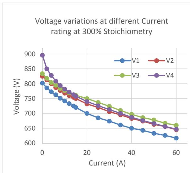
Figure 3. Cell voltage variation from OCV- 60A load for the 4 cell stack at 300% air Stoichiometry
