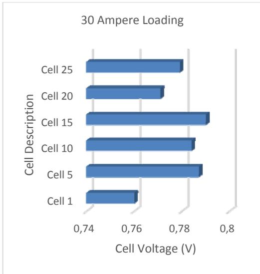
Figure 7. Ballard Mark 9™ cell to cell variation at 30 amps.
