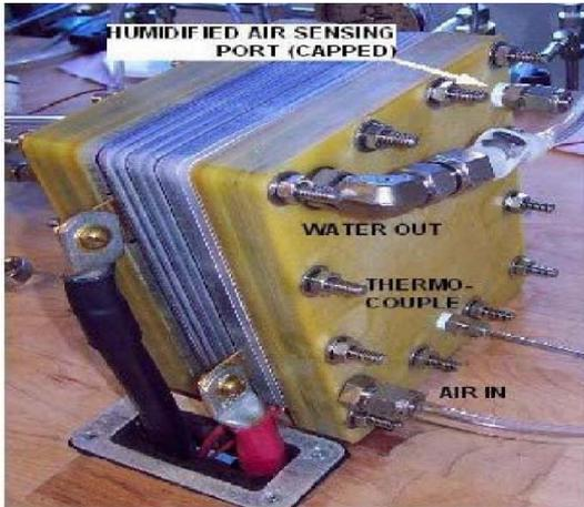
Figure 1(a) the air side of the SERC -140 stack
