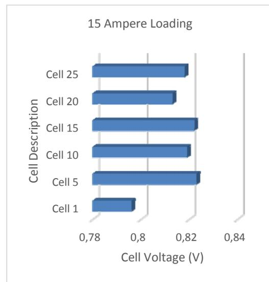
Figure 6. Ballard Mark 9™ cell to cell variation at 15 amps.
