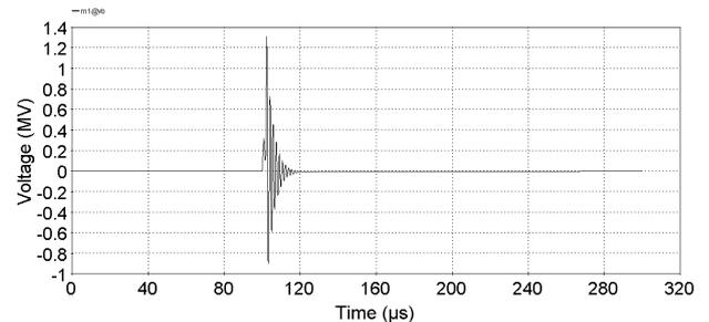
Fig. 4. Overvoltage at the wind turbine.
