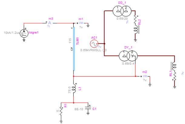
Fig. 2. EMTP-RV circuit.
