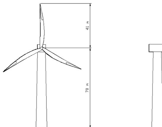
Fig. 1. Dimensions of the wind turbine.
