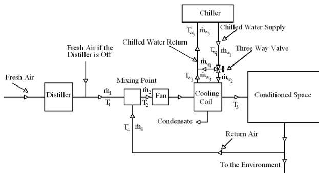
Fig. 1: Schematic of the solar distiller unit and air-conditioning integrated system
