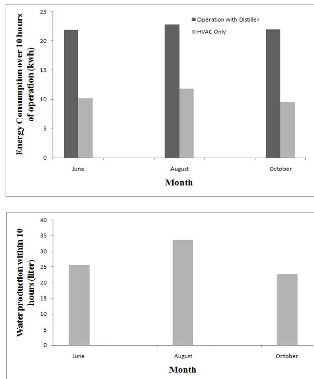
Fig. 3: (a) the optimized total energy consumption bar chart in kWh for the 10 hours of operation when the distiller is operated and when it is not operated for the different months and (b) The amount of water condensate over 10 hours when the distiller is not operated with the HVAC system.
