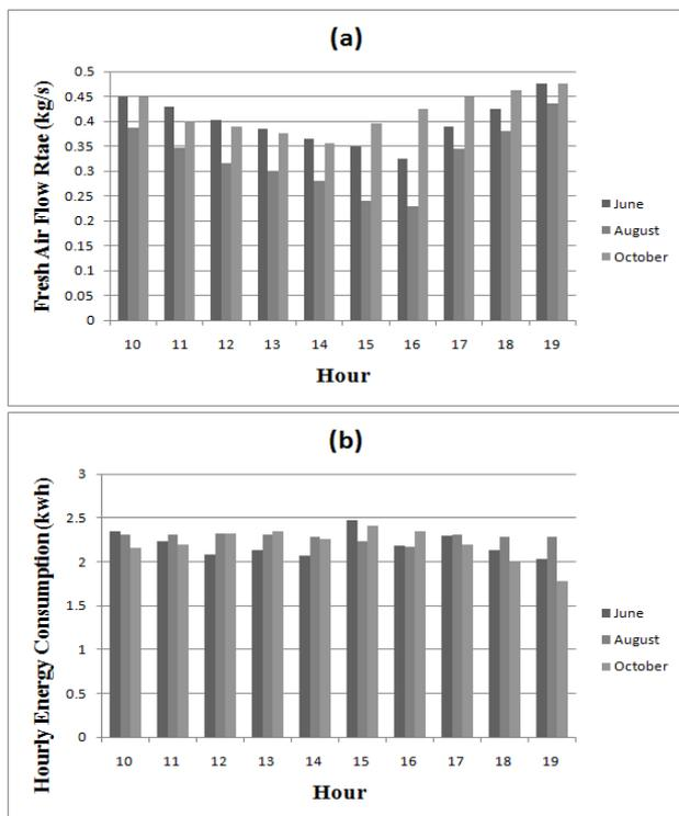
Fig. 2: (a) optimized fresh air flow rate design variable for the hours of operation for the studied months (June, August & October) and (b) the optimized hourly energy consumption bar chart in kWh for the different three months as a function of the hour of the day.
