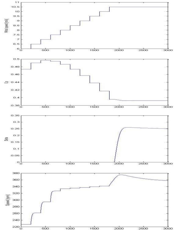
Fig. 7. Torque and speed control upon wind increase
