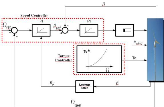
Fig. 6. Block diagram of the GARBI-150 control system
