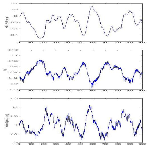
Fig. 8.  $C_p$ , pitch angle and rotor speed using control speed control strategy
