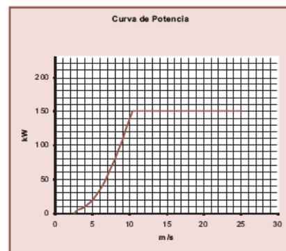
Fig. 1. Wind turbine power curve
