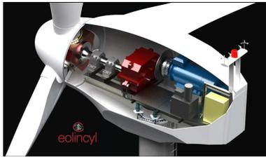
Fig. 2. GARBI-150. Wind Turbine Scheme
