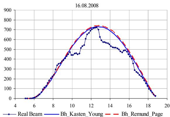
The turbidity factor values, recommended by the technical literature for the Braşov area (these values do not take into consideration at least the urban condition of Braşov), do not correspond to the real values calculated on the basis of the recorded meteorological data.
