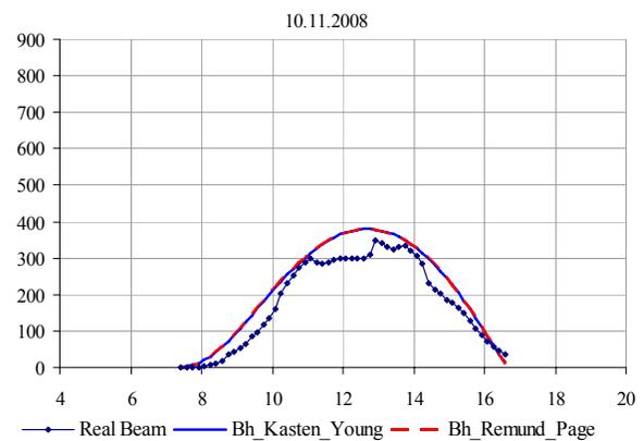
Fig.6. Theoretical simulation of the beam horizontal irradiance for Braşov Area
