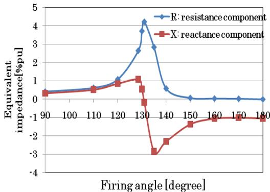
Fig.2. Experimental results of Impedance characteristic of TCSC
