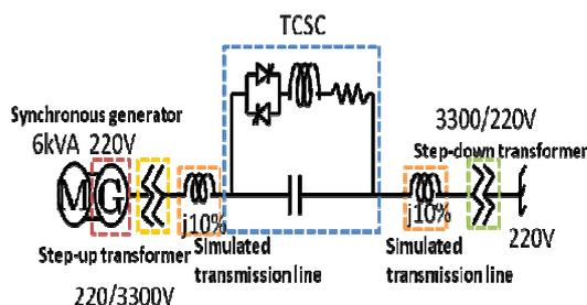
Fig.3. Single machine infinite bus system
