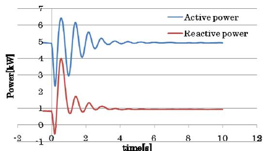
Fig.4 Power oscillation with TCSC
