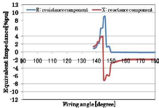
Fig.6 Impedance Characteristic by experiment
