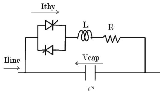
Fig.1. Configuration of TCSC prototype
