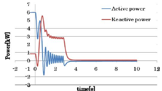
Fig.5 Power oscillation without TCSC
