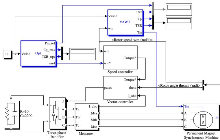
Fig. 4. The implemented simulink model of WGS
