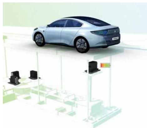
Fig. 3. Quickdrop charging system
