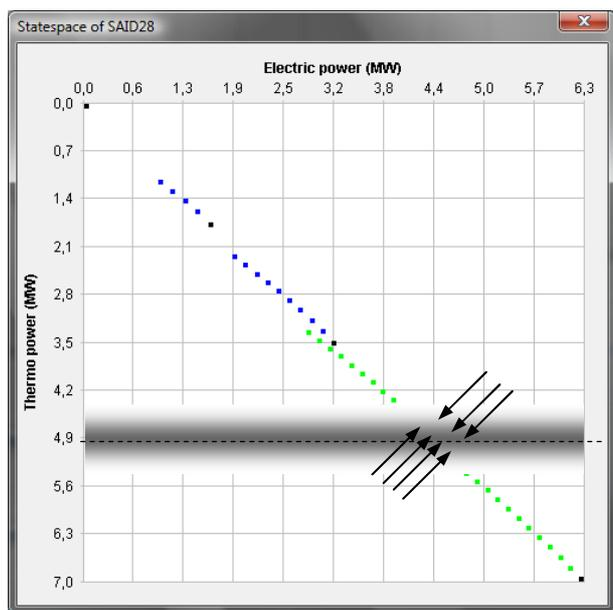
Fig.1 Method of state-space (DG with 4 gas-engines). [4]
