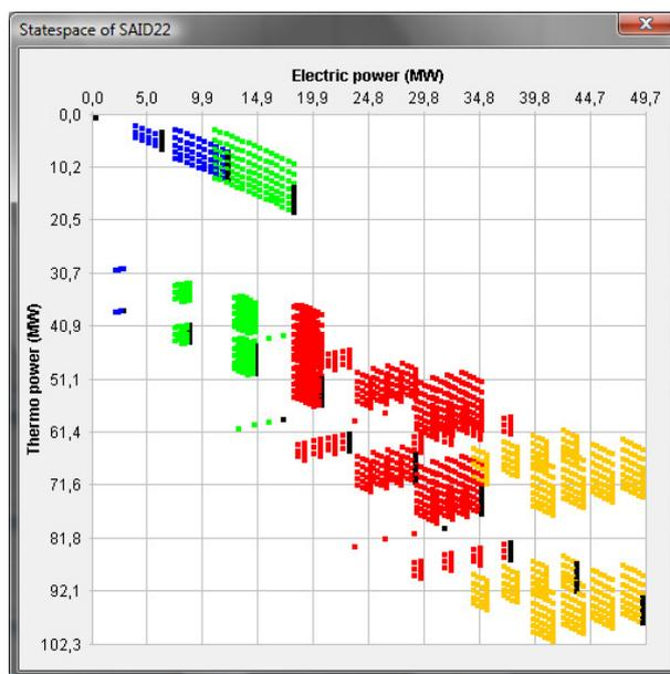
Fig.2 A more complicated state-space (DG has gas-engines, stoker and steam-turbines also)
