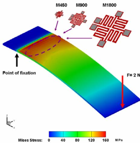
Fig. 5. Stress distribution in loaded beam, z-axis is magnified to see the bending
