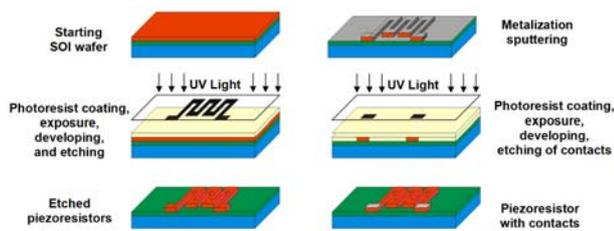
Fig. 7. Technological process of SOI sample production
