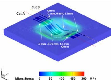
Fig. 2. Mechanical analysis - membrane deflection under applied pressure, and sensitivity analysis of meander and straight resistor
