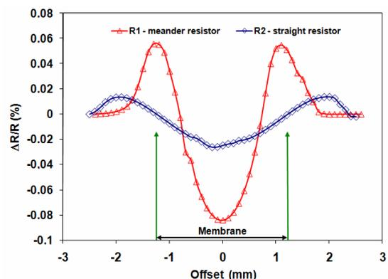
Fig. 4. Piezoresistive sensitivity analysis of the meander resistor (R1) and the straight resistor (R2) and their dependence on offset
