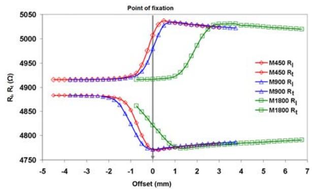
Fig. 7. Change in meander resistance in dependence on position with respect to point of fixation (Offset = 0 mm)
