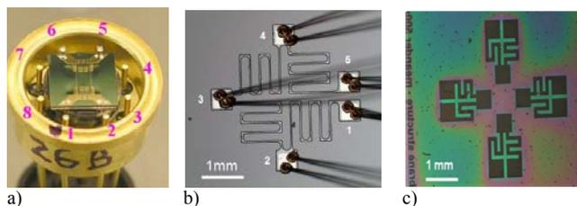
Fig. 8. a) structure of membrane pressure sensor with NiCr piezoresistive layer; b) SOI strain gauges; c) strain gauges with NCD layers
