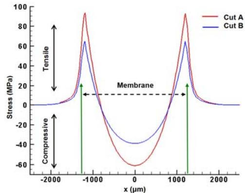
Fig. 3. Stress distribution along the centre line of the membrane (Cut A) and off the centre (Cut B)
