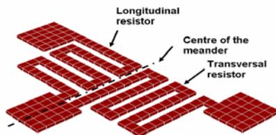
Fig. 6. Meshed 3D model of the structure M450, with longitudinal and transversal meander
