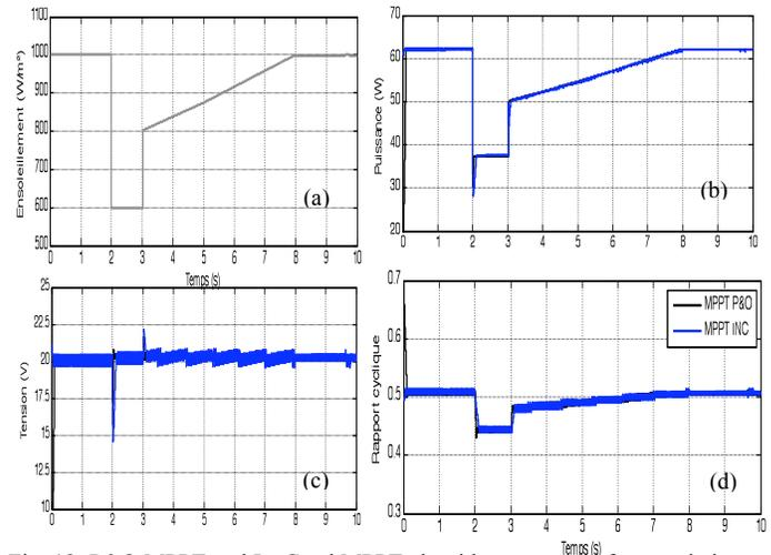
Fig. 18: P&O MPPT and IncCond MPPT algorithm responses for a variation of illumination and a constant temperature of 25°C: (a) variation of the irradiation, (b) PVG power, (c) PVG voltage, (d) duty cycle.
