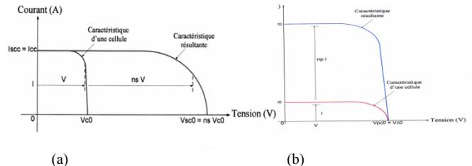
Fig. 7: I-V characteristic of a photovoltaic module with cells in (a) series associating and in (b) Shunt associating.
