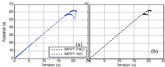
Fig. 17: Characteristic curve P(V) of (a) P&O and (b) IncCondMPPT controllers for a change in the temperature from 25°C to 50°C at a fixed irradiation equal to 1000W/m<sup>2</sup>.
