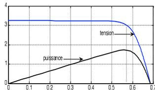
Fig. 2: I-V and P-V cell Characteristics.
