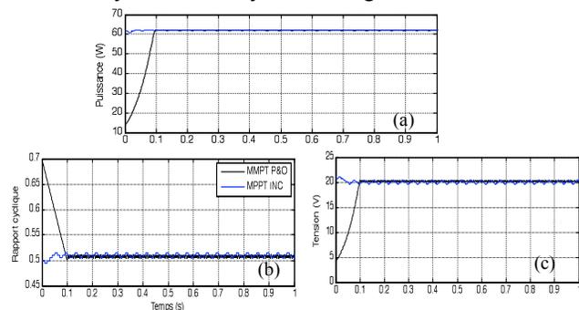
Fig.13: Variation of (a) the power, (b) the voltage of the module and (c) the duty cycle of two controllers P&O MPPT (grey line) and IncCond MPPT (blue line) for  $T = 25^{\circ}\text{C}$  and  $G = 1000\text{W}/\text{m}^2$ .
