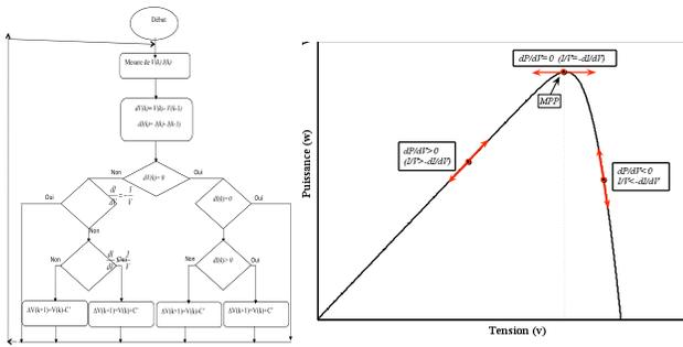
Figure 11: Flow chart algorithm of IncCond MPPT and principle show in a P-V characteristic.
