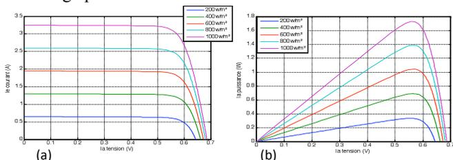
Fig. 5: Irradiation influence on PV cell characteristics at constant temperature  $T=25^\circ C$ . (a) I-V curves, (b) P-V curves.
