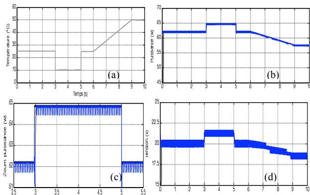
Fig. 19: P&O MPPT and IncCond MPPT algorithm responses for a variation of temperature and a constant illumination of  $1000\text{W/m}^2$ : (a) variation of the temperature, (b) PVG power, (c) Zoom in PVG power, (d) PVG voltage.
