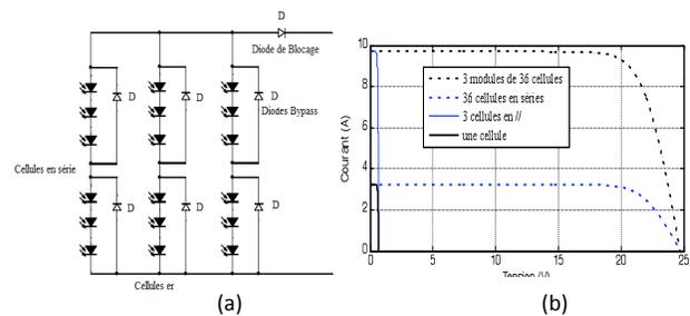
Fig. 8: (a) Scheme of a photovoltaic generator and (b) its I-V curve compared with I-V curves for modules and cells.
