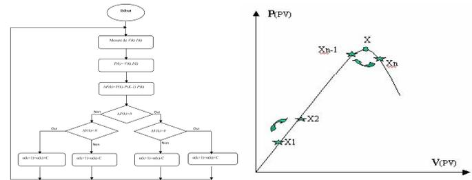
Fig. 10: Flow chart algorithm of perturb-and-observe (P&O) MPPT and principle show in a P-V characteristic.
