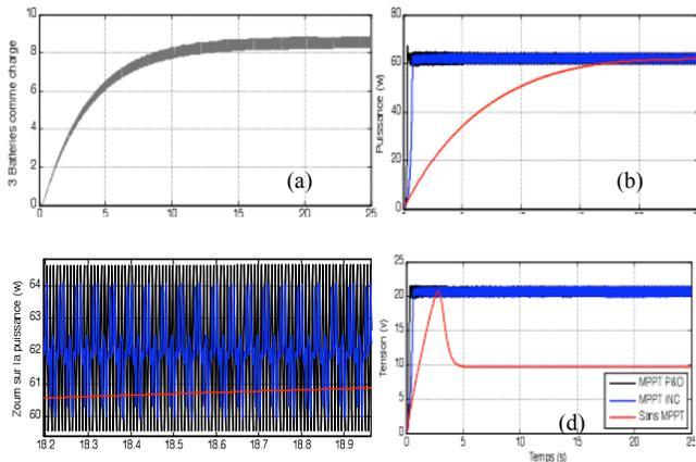
Fig. 16: Influence of the load (a) of three batteries according to time on: (b) power, (c) zoom on power curve, (d) voltage, without (red line), with P&O (grey line) and IncCond MPPT (blue line) controllers.
