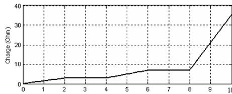
Fig. 14: Dynamic resistor load. The variation of the resistor is shown according to time.
