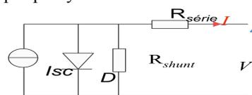
Fig. 1. Equivalent circuit of a photovoltaic cell
