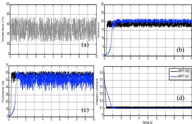
Figure 20: P&O MPPT and IncCond MPPT algorithm responses for a random variation of temperature: (a) variation of the temperature, (b) PVG power, (c) PVG voltage, (d) duty cycle.
