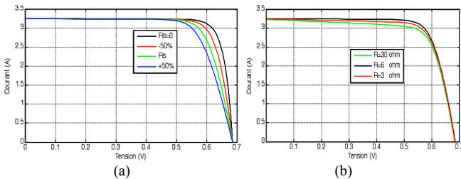
Fig.3: Influence of: (a)  $R_s$  and (b)  $R_{sh}$  on I-V characteristic.
