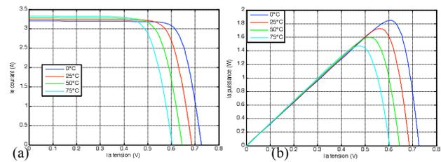
Fig.6: Temperature dependence of the P-V characteristics at constant irradiation  $E=1000 w/m^2$ . (a) I-V curves, (b) P-V curves.
