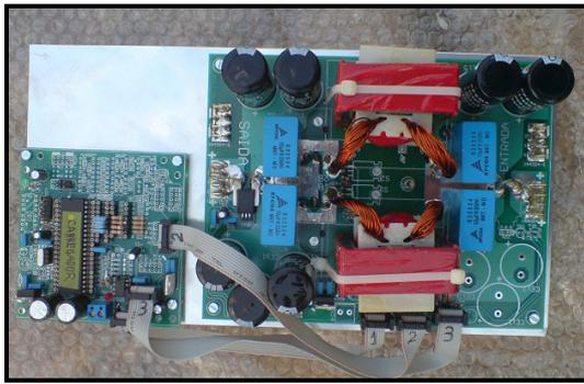
Fig. 6. Battery charger prototype.
