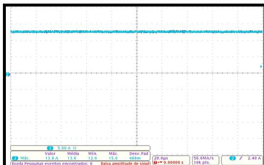
Fig. 13. Input current (into the battery) (5A/div).
