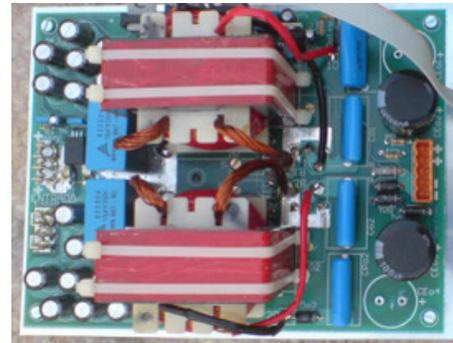
Fig. 9. Top view of the boost high-gain.
