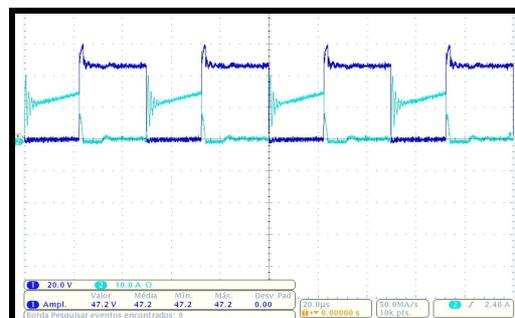
Fig. 11. Current through L1 (CH2) and voltage across the power switch (CH1). (20V/div), (10A/div)
