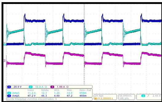
Fig. 12. Current through L1 (CH2), L2 (CH3) and voltage across the power switch (CH1). (20V/div), (10A/div and 1A/div ).
