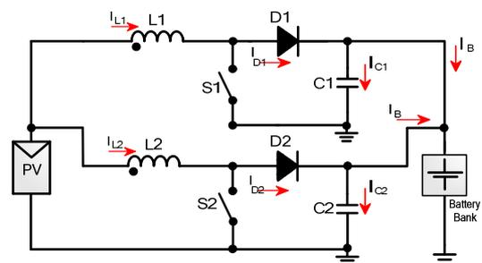
Fig. 5. Basic electric schematic of the battery charger.
