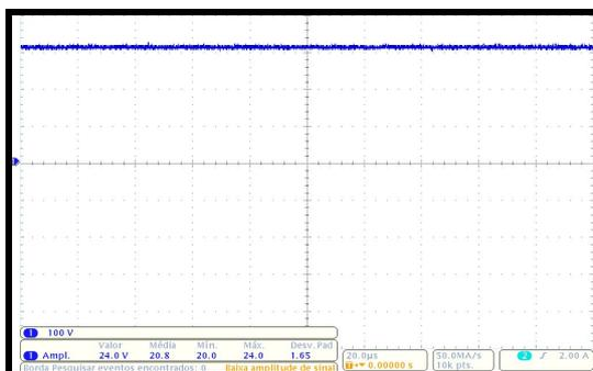
Fig. 14. High gain boost converter output voltage (100V/div).
