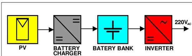
Fig. 2. System with DC/AC converter, output: 220 V<sub>Ac</sub>.
