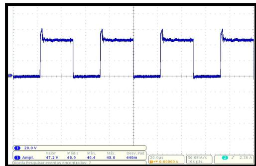
Fig. 10. Voltage across the power switch (with load) (20V/div).
