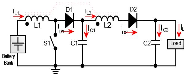
Fig. 7. Electric schematic of the boost converter.
