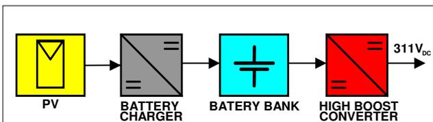
Fig. 3. System with DC/DC converter, output: 311 Vdc.
