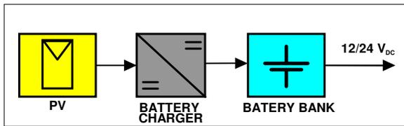
Fig. 1. Simple DC system, output: 12/24 Vdc.
