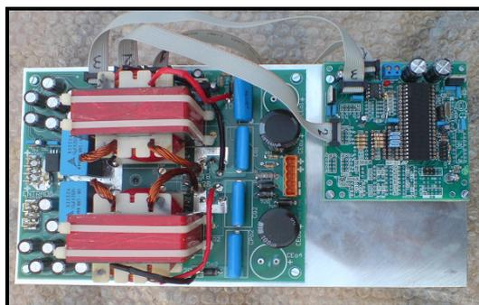
Fig. 8. Boost converter prototype.
