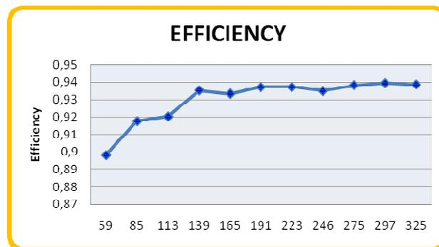
Fig. 15. High gain boost converter efficiency.
