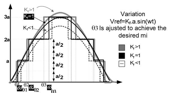
Figure 5: Flexible method of sinusoid reference used to obtain the optimized THD.
