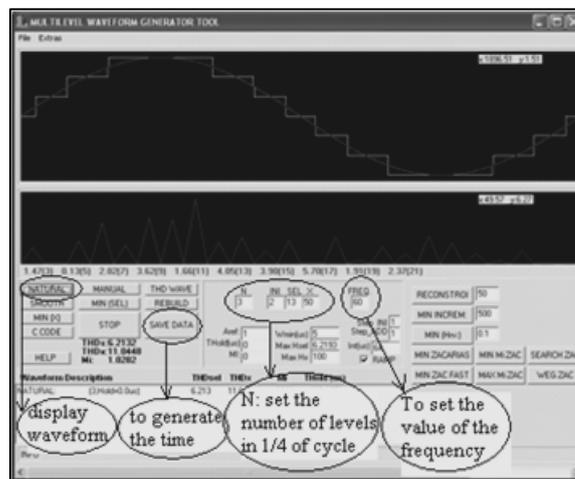
Figure.7 Environment interface: sine wave treatment unit, generator of the transition times of the sine staircase levels.
