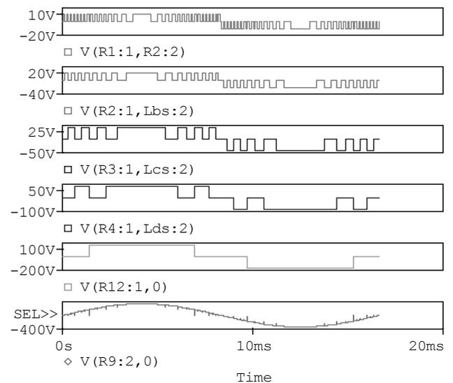
Fig.11: Waveforms from the first to the fourth graphic, in the output, from first to last cell L (fig. 11). Last graphic is a sine curve, with output voltage in linear load (R).
