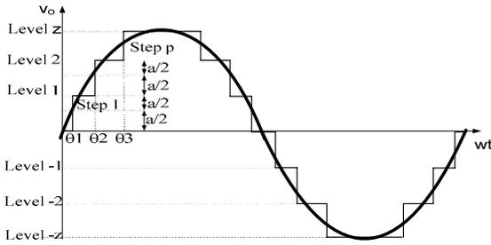
Figure 1: Multilevel waveform.
