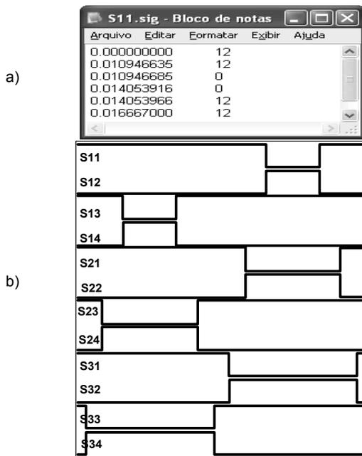
Fig.9: b) File .sig imported by through the VPWL\_FOREVER function; c) monitor screen the driven pulses of the switches.
