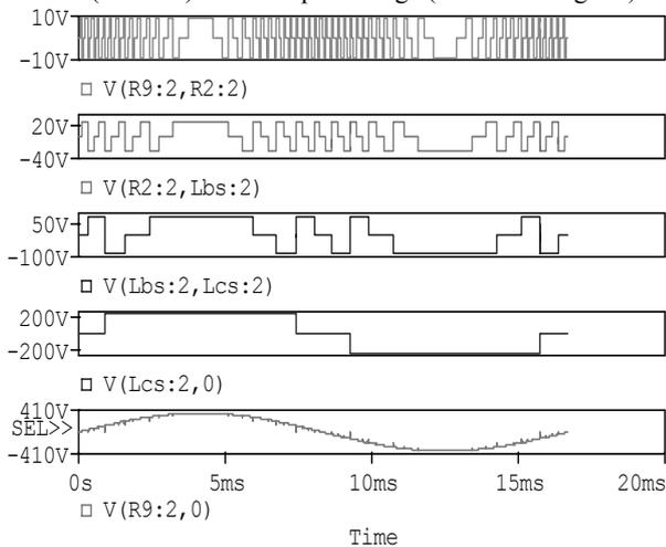
Fig.13 The first to the fourth graphics show voltages in secondary windings, respectively, from first to last using the secondary configuration ternary. Last graphic: output voltage waveform, operating in 220VA 1kVA.
