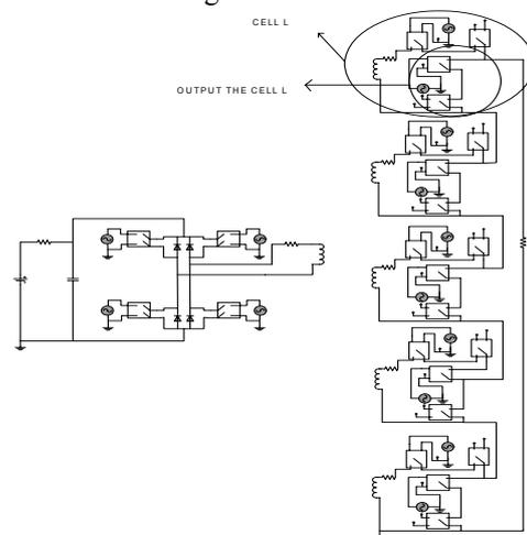
Fig.10 Simulate inverter employed by [1] with 63 levels ( $+z$  to  $-z$ ) in output voltage, simulated with input voltage of 48V, and output 220-1kVA (waveform: fig.12).
