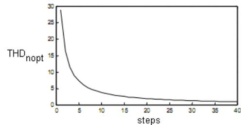
Figure 2: THD output voltage depending on the number of steps in  $1/4$  cycle of sine.
