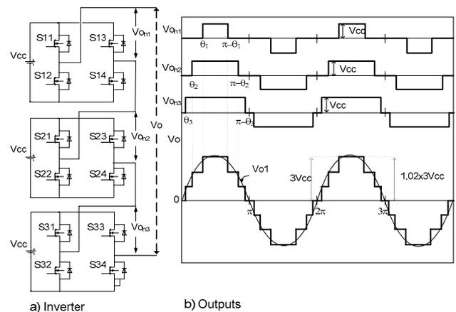
Figure 3: From top to bottom, the output voltage in the cells ( $V_{o_{h1}}$ ,  $V_{o_{h2}}$  and  $V_{o_{h3}}$ ) fourth cycle and the last graph in the output voltage of the inverter.
