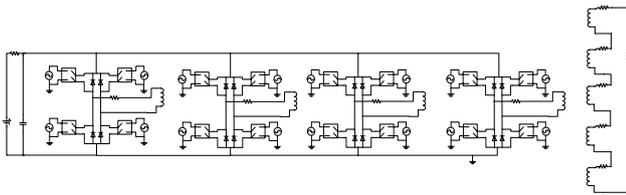
Fig.12: Topology simulated with the ternary configuration with 81 levels (+z to -z) in the output voltage (waveform: fig. 14).
