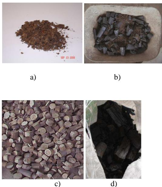
**Figure 02:** Biomass gasification used in: a) Cake of Coconut Macaúba, b) Cake of Coconut Macaúba mixed with charcoal, c) Eucalyptus firewood e d) Charcoal.
