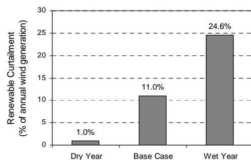
Fig. 8. Impact of different hydrological regimes in the needs for renewable generation curtailment
