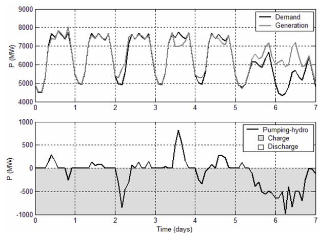
Fig. 7. Contribution of the pumping-hydro operation to the power system balance along one week of the base case scenario
