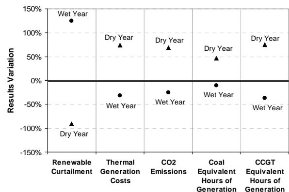
Fig. 10. Impact of different hydrological regimes in the power system operation parameters, in the year 2011
