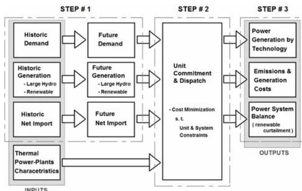
Fig. 1. Diagram of the proposed methodology
