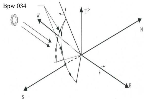
Fig.3. Numbering and Orientation of eight photodiodes
