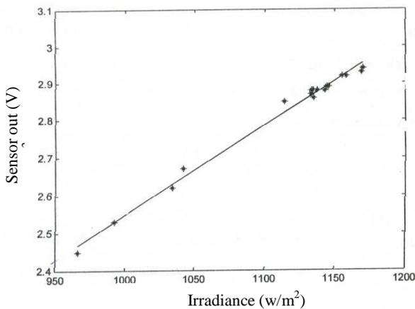
Fig 2: Calibration of the conditioning circuit
