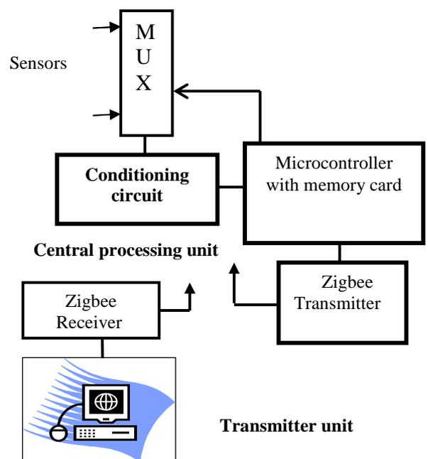
Fig 1. Block diagram of the data acquisition system.
