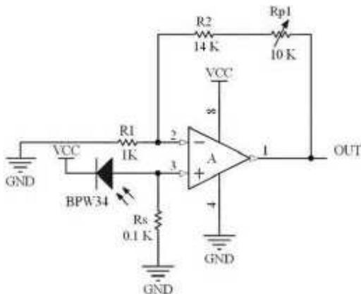
Fig. 1 conditioning circuit for each single photodiode.
