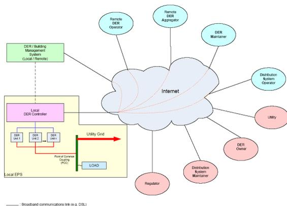
Figure 3. Example on the Communications System Architecture for DER
