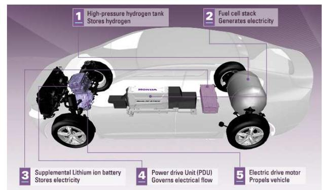
Fig. 7. Fuel Cell Electric Vehicle (FCEV)
