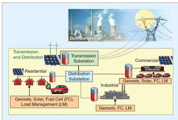
Figure 6. Power system with integrated central & distributed energy resources.
